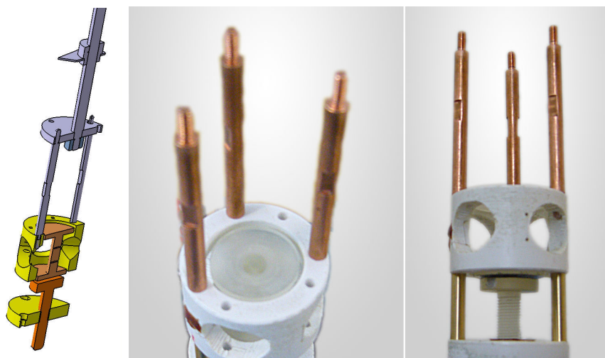
FIGURE 4.5: The "plastic sample holder": schematic view (left) and the capacitive sensor (right).
