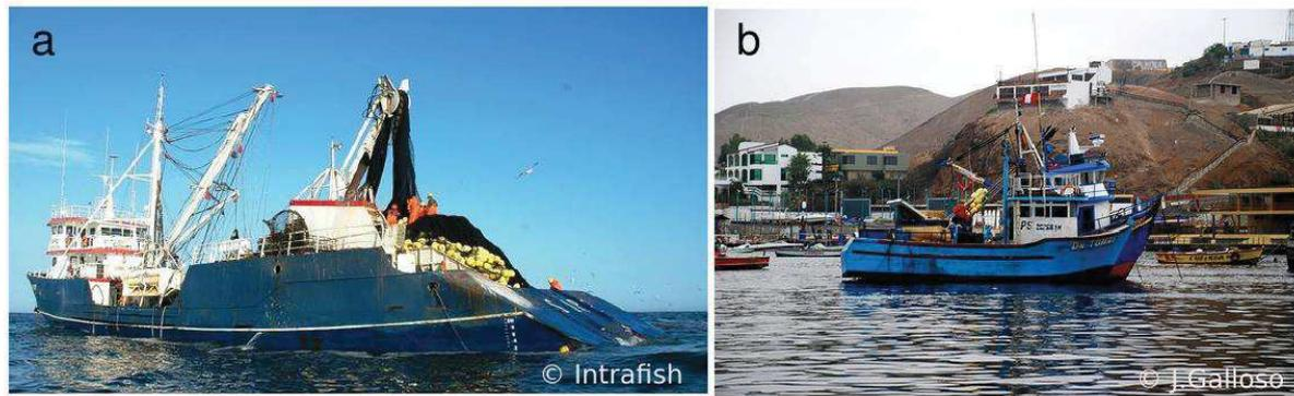
Figure 1.12. Purse-seiners used to catch anchovy, a) “industrial” purse seiner with a steel hull and b) “artisanal” purse-seiner with a wooden hull.
