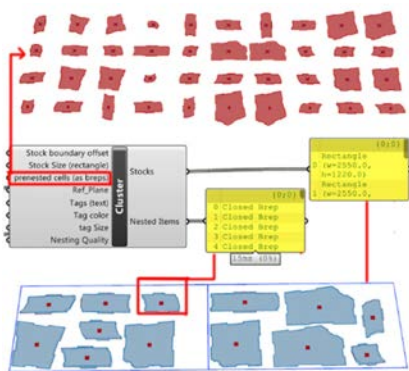
Figure 214. Pre-nested items are once again reoriented into stocks by means of reference plane. Nesting gaps can be adjusted with the nesting quality value
