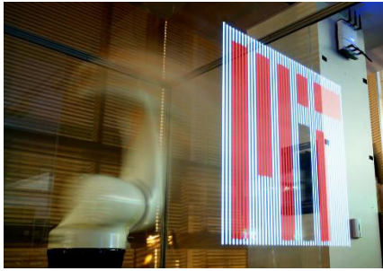
Figure 115. Light Painting. An image drawn in space through robotic kinematics. The drawn light pattern is captured through long exposure photography. On: http://matter.media.mit.edu/tools
