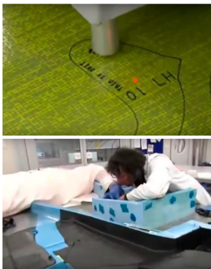
Figure 113. Manufacturing carbon fiber pieces requires a mixture of techniques that go from 2D laser-cutting to die forming. Top. A component for a F1 race car wing is cut with a 2D laser CNC machine. Bottom. Pieces for the same wing are being put in place into a die so they acquire a specific form. Carbon fiber is later hardened with an epoxy resin and cured in an autoclave. (Daldry, 2012)
