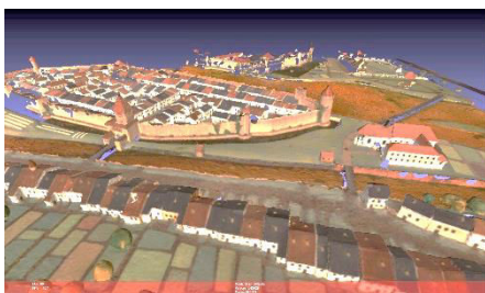
Figure 69. 3D model of the town of Epinal-France. This survey model is taken from a scale model of the town's ancient ramparts. New scanners and software allow for collecting data including not only geometric but texture information out of the surveyed model. C.R.A.I 2015.
