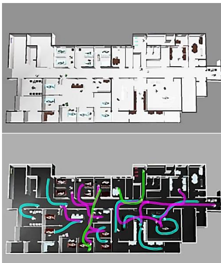
Figure 76. Human behavior simulation. Based on a BIM model, a simulation allows to estimate how crowded a space can get thus helping to stablish whether rooms and corridors are big enough in case use intensity suddenly increases. Bnai Zion Medical Hospital, Y.Kalay, 2012. Top On: youtube.com/watch?v=i05WVWUprmyU-
