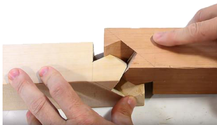
Figure 141. Top. Scarf-like Japanese beam-joint. (Building Channel, 2016) Bottom. Three-way Japanese interlocking joint (Wandel, 2015).
