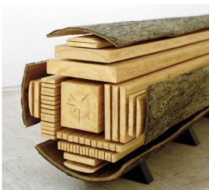
Figure 136. Dimension lumber as obtained from sawn logs. On: thedesignconfidential.com
