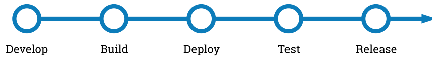
Figure 2.3 – Overview of a continuous deployment pipeline, defining all stages from development to release. Tests range from unit tests, to integration and acceptance tests. Existing tools for continuous integration, development and delivery include Jenkins 1 , Travis CI 2 , GitLab CI 3 , Circle CI 4 , and Codeship 5 .
