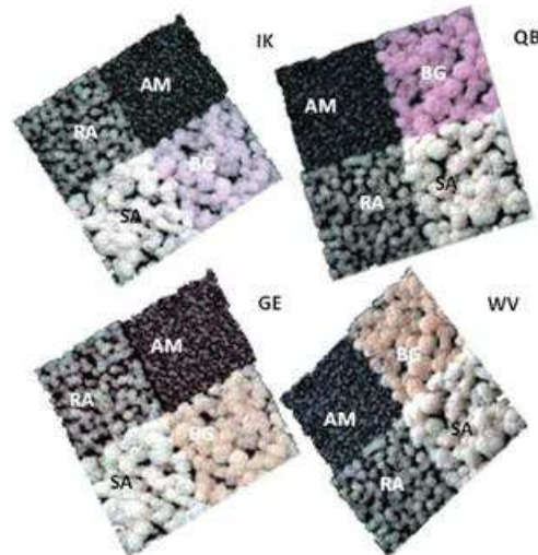
Fig. 5. 100x100m simulated satellite images with a sun zenith angle of 20° at viewing zenith angles given in table 1 (pixel size=50cm).
