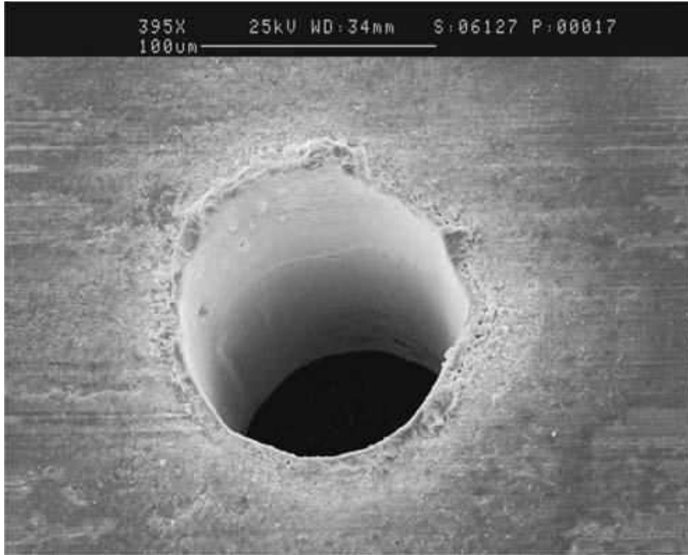
Figure 1.7: SEM images of laser-trepanned holes on copper,(Tünnermann, 2009)
