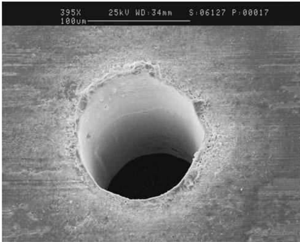
Figure 1.7: SEM images of laser-trepanned holes on copper,(Tünnermann, 2009)
