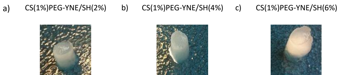
Fig. 6. Photographs of crosslinked CS/PEG sponges of which PEG was a mixture of PEG-YNE (tetra alkyne) and PEG-SH (bis thiol) ([SH]/[YNE] ratio of 1.3). Polymer percentage are expressed in w/v.
