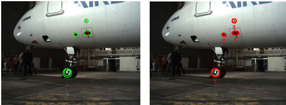
(a) Robot near the aircraft. Ellipse extraction with EDCircles. (b) After postprocessing (merging ellipses).
