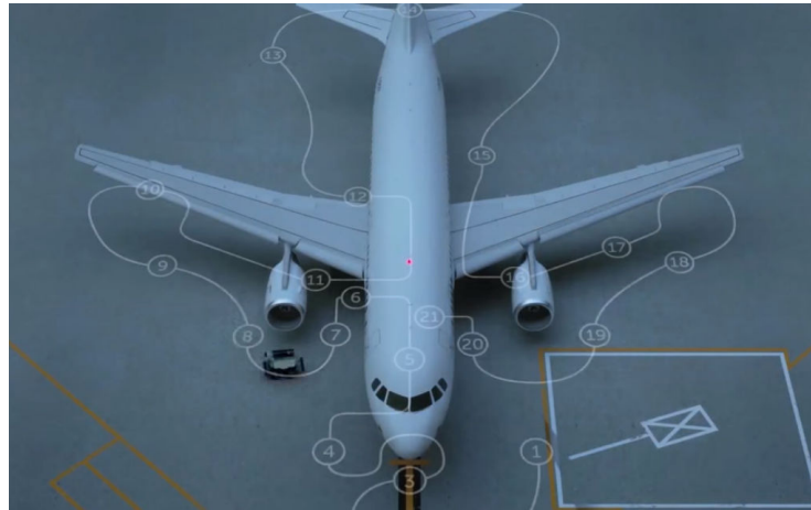
Figure 1.2: Predefined inspection trajectory: 'walk around'.
