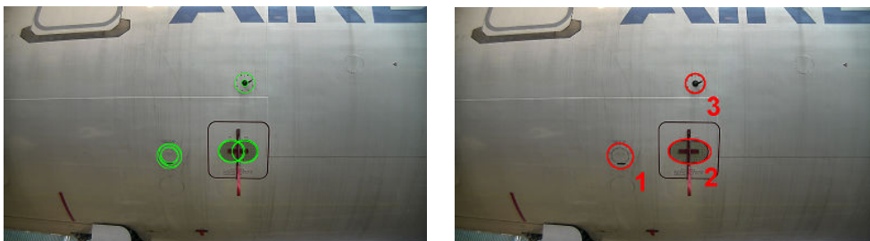
(a) Robot in the inspection checkpoint. Ellipse extraction with EDCircles. (b) After postprocessing (merging ellipses).
