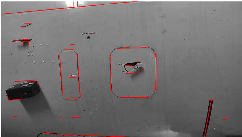
(b) Set of segments after merging and filtering. In this case only nearly horizontal or vertical segments are kept.
