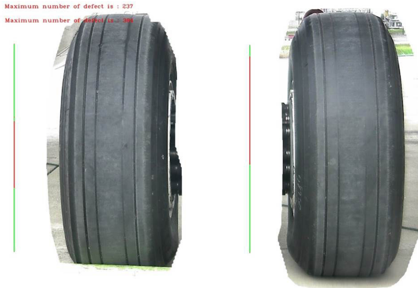
Figure 3.87: Final tire inspection result
