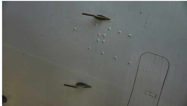
Figure 3.49: Two Pitot probes on Airbus A320 aircraft. Verification type: INTACT/BROKEN . Both probes in the image are intact (negative case).
