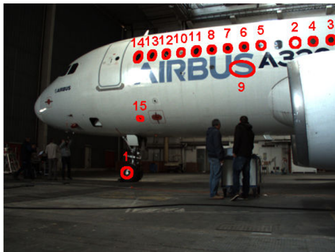
(c) Ellipse detection in the sensed image (EDCircles and our postprocessing step).
