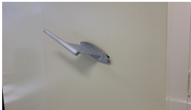
(b) Pitot printed in 3D from the CAD model.
