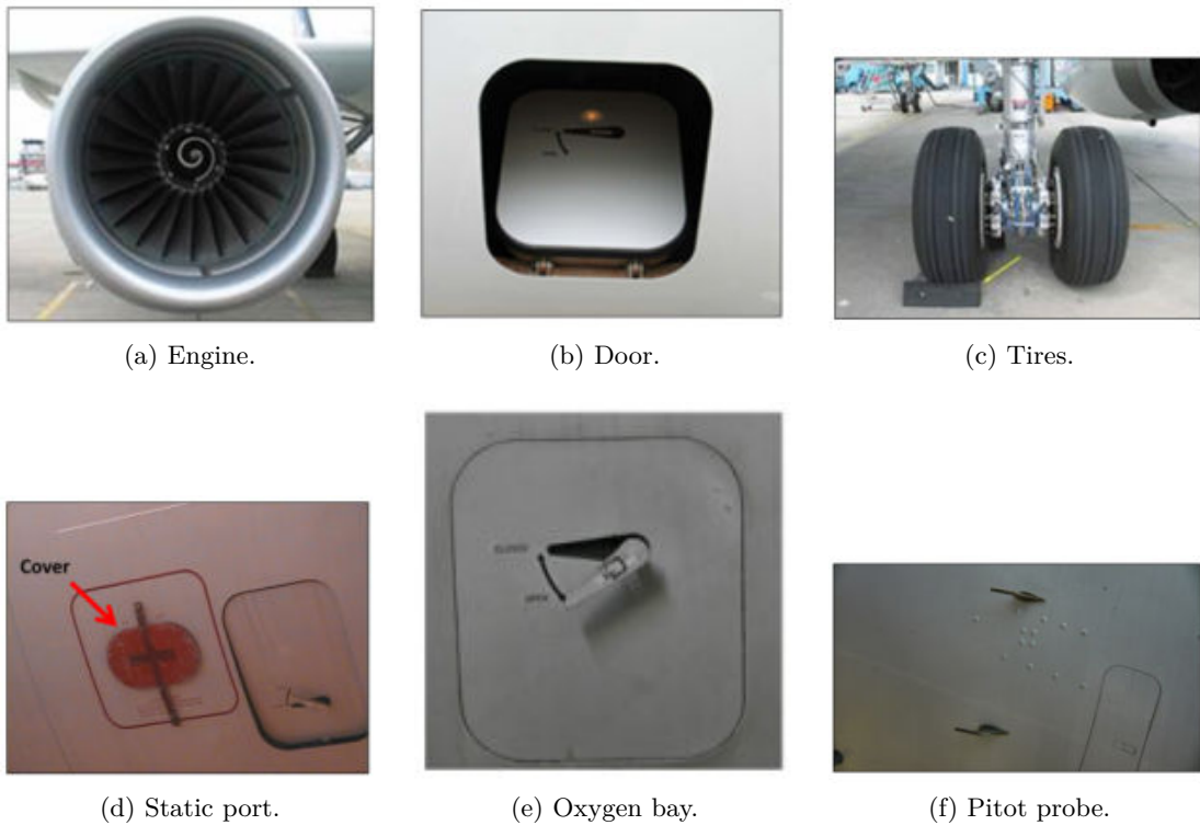
Figure 1.3: Examples of items to be inspected.
