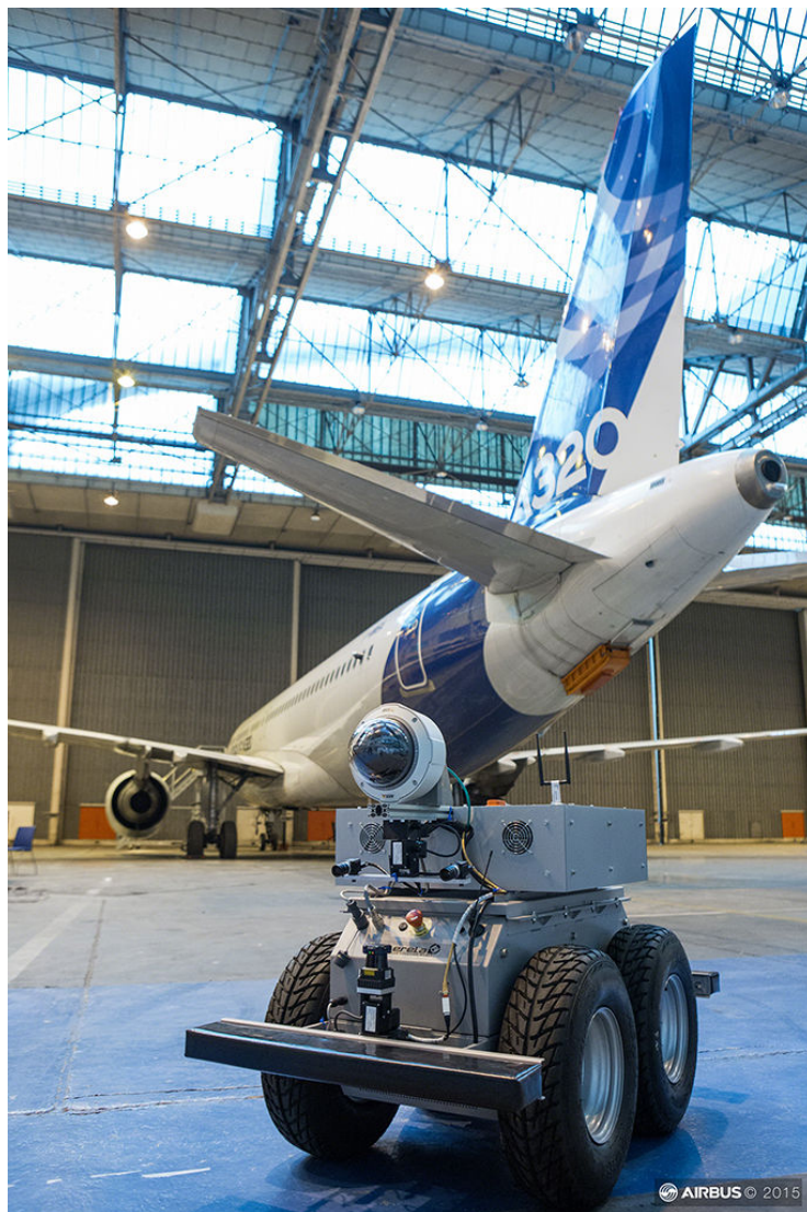
Figure 2.1: PTZ camera mounted on the robot.
