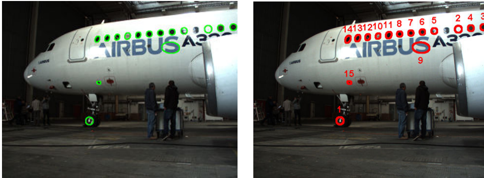
(a) Robot far from the aircraft. Ellipse extraction with EDCircles. (b) After postprocessing (merging ellipses).
