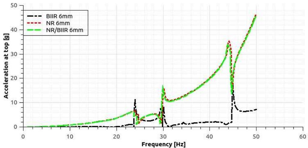
Figure 4.20: Acceleration quantity with 6 mm thickness of rubber insert at node 2465
