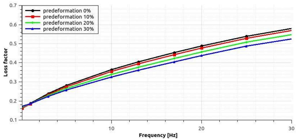
Figure 2.46: Loss factor frequency and predeformation dependence: BIIR
