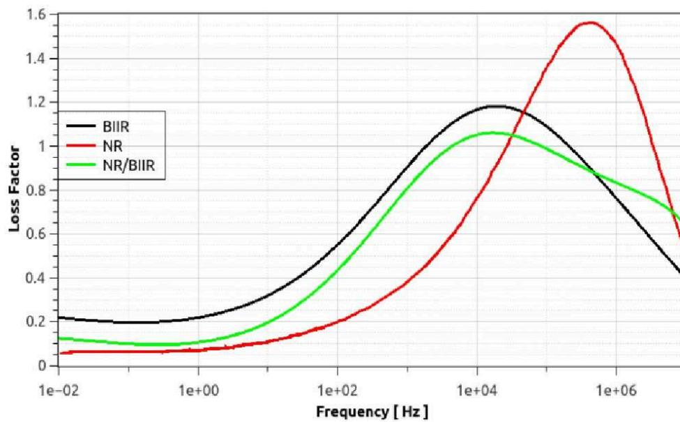
Figure 2.42: Loss factor Master curves, comparison of the three materials
