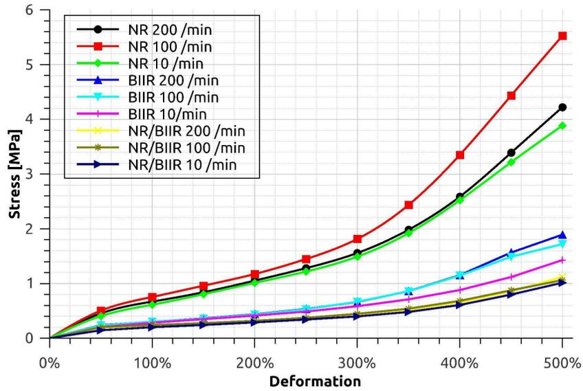
Figure 2.16: Non-equilibrium tension stress response at different strain-rates
