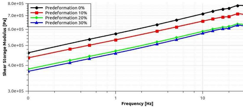
Figure 2.45: Shear modulus frequency and predeformation dependence: NR/BIIR
