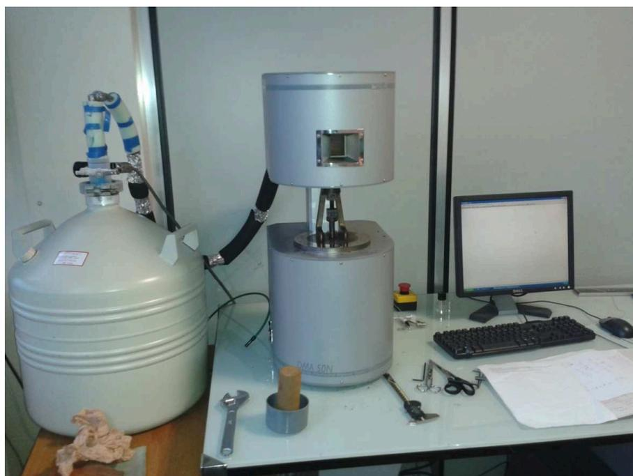
Figure 2.5: Metravig DMA 50N testing machine
