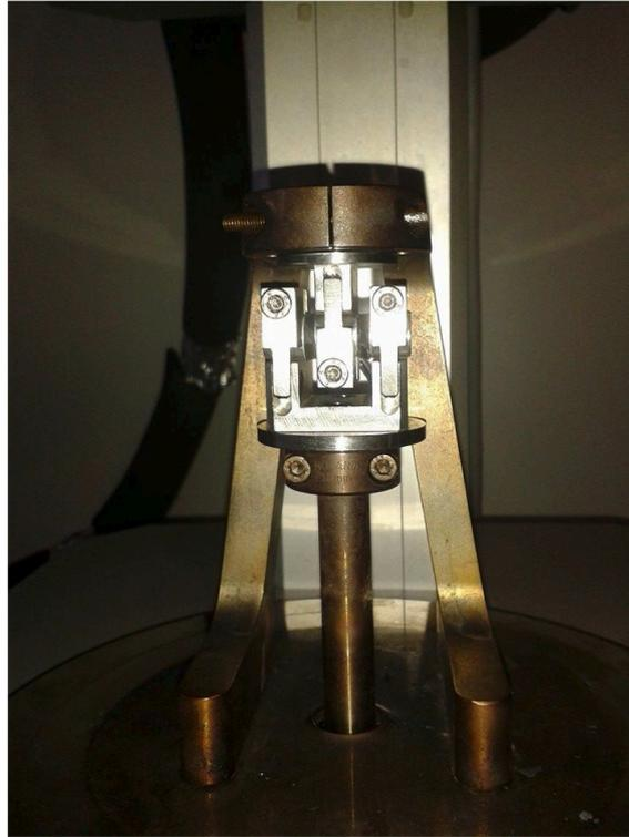
Figure 2.11: DMA shear specimen holder
