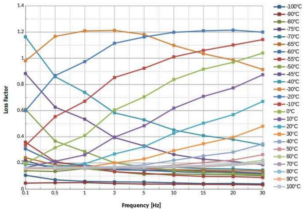
Figure 2.36: Isothermal Loss factor: BIIR
