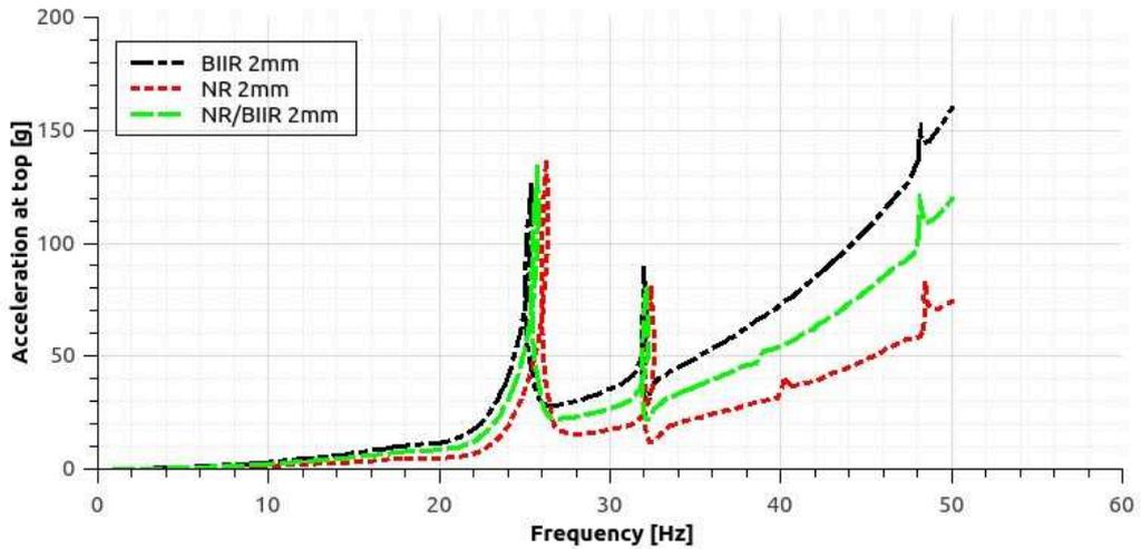
Figure 4.16: Acceleration quantity with 2 mm thickness of rubber insert at node 2465
