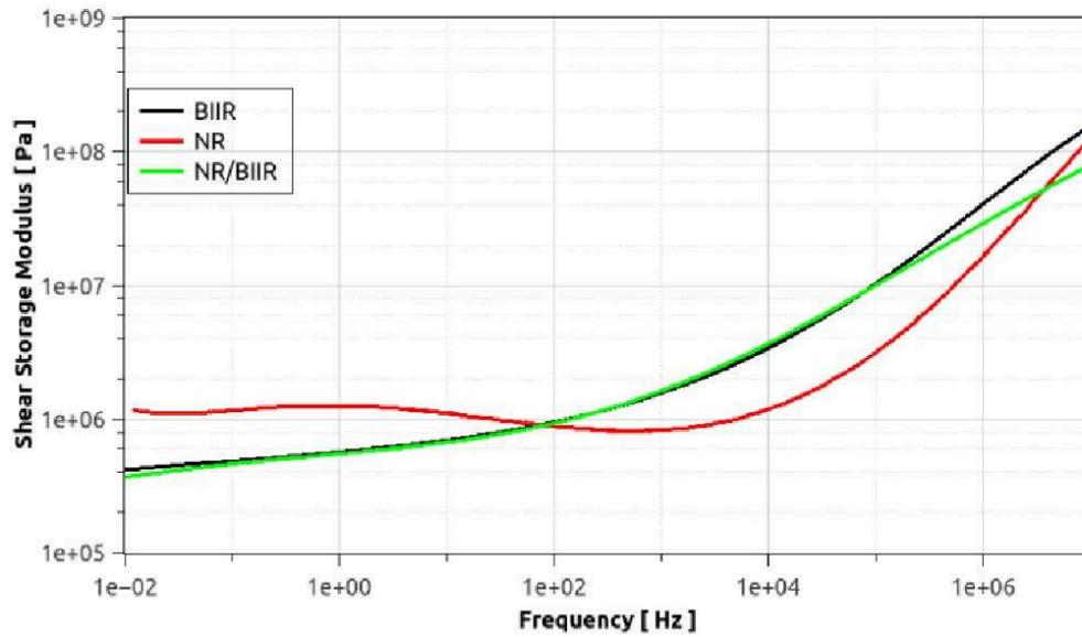
Figure 2.41: Shear storage modulus Master curves, comparison of the three materials
