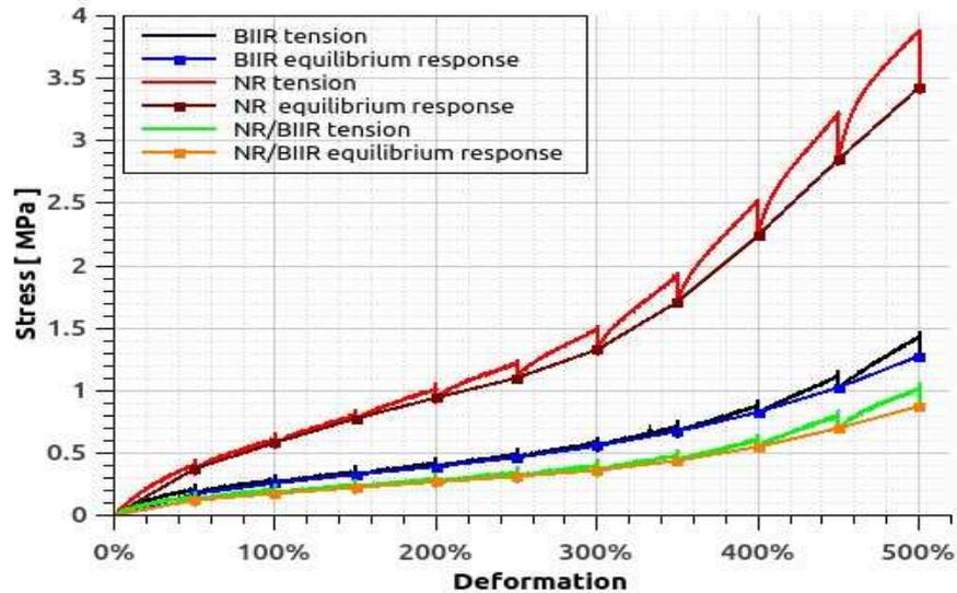
Figure 2.17: Definition of the equilibrium stress-strain curve for the tension mode
