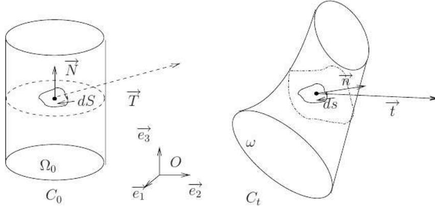
Figure 1.9: Stress vectors at different configurations
