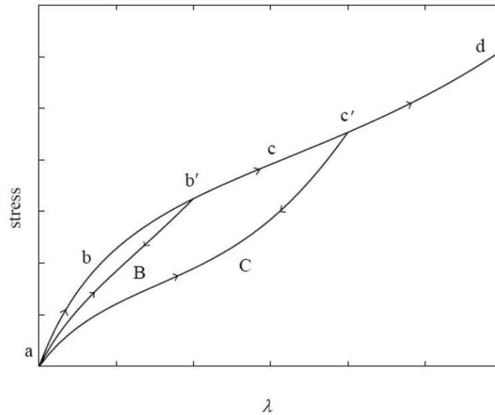
Figure 1.6: Cyclic loading with evident Mullins effect [24]
