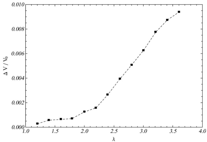
Figure 1.2: Volume change of filled rubber materials [15]
