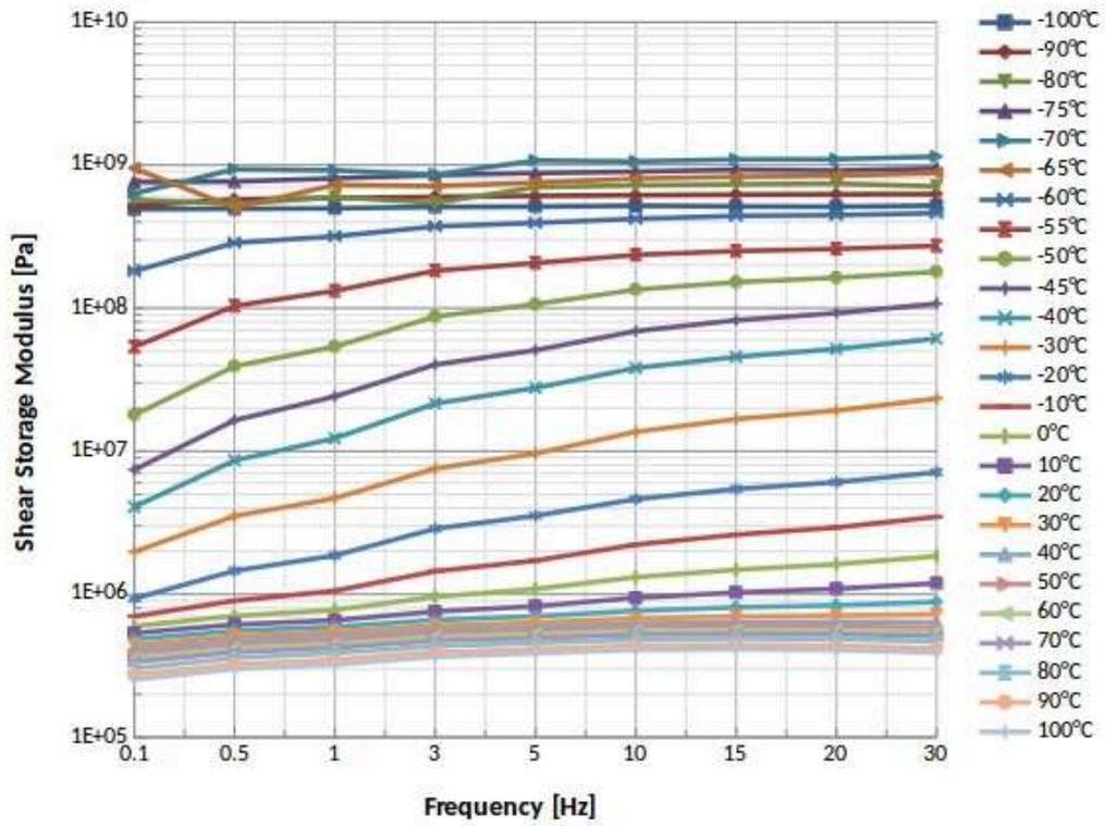
Figure 2.39: Isothermal Shear storage modulus: NR/BIIR
