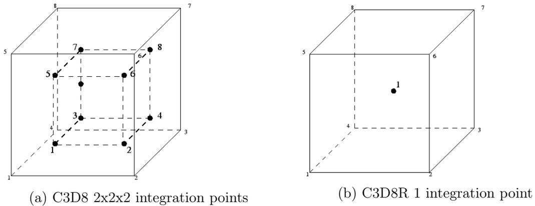
Figure 4.8: Mesh elements: C3D8 vs C3D8R
