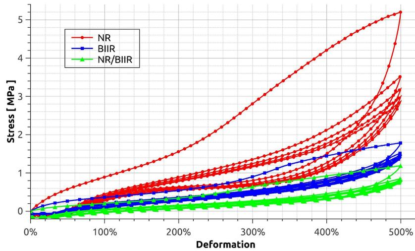
Figure 2.14: Uniaxial tension cyclic loading
