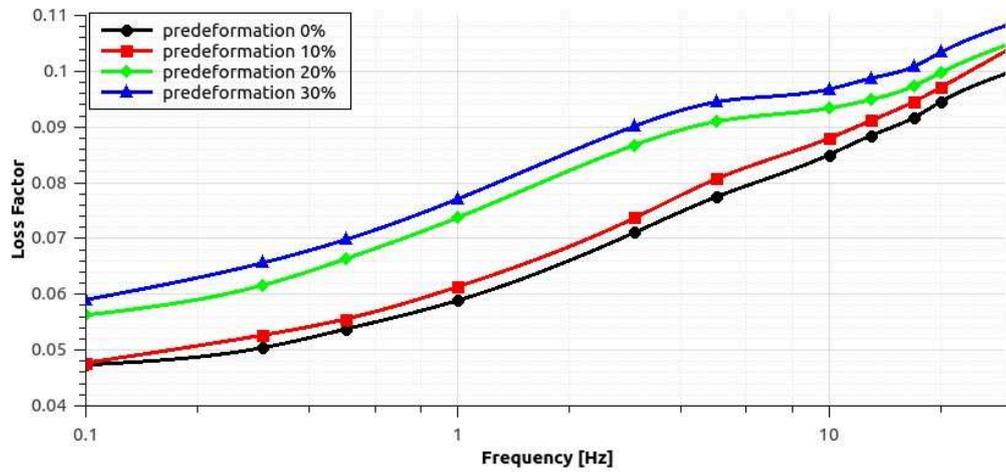
Figure 2.47: Loss factor frequency and predeformation dependence: NR
