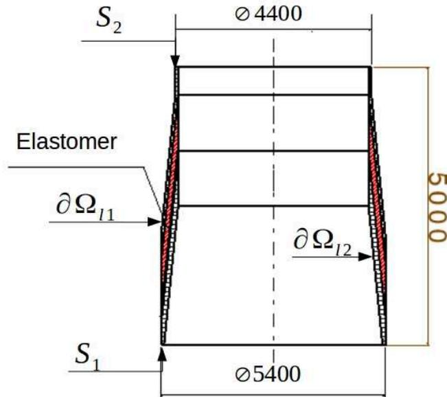
Figure 4.7: Inter-Stage 2/3 geometry
