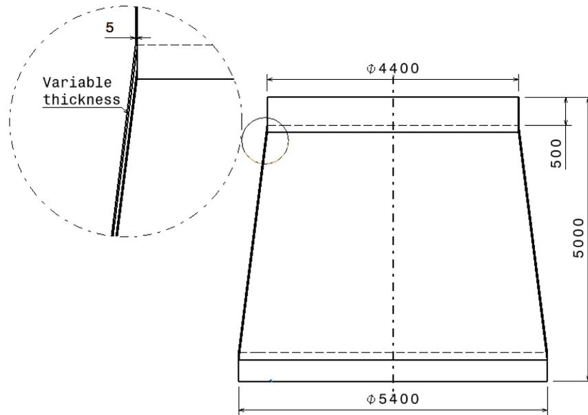
Figure 4.4: Proposed Inter-Stage 2/3 geometry
