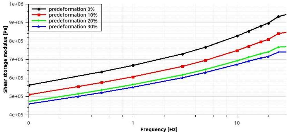
Figure 2.43: Shear modulus frequency and predeformation dependence: BIIR
