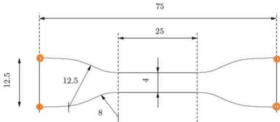
Figure 2.8: H2 Specimen dimensions in mm
