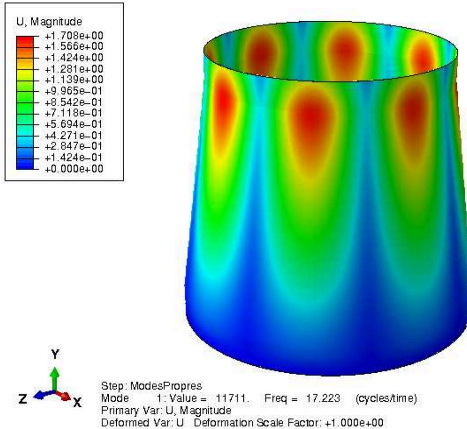
Figure 4.11: 1<sup>st</sup> fundamental lateral mode shape: Damped BIIR
