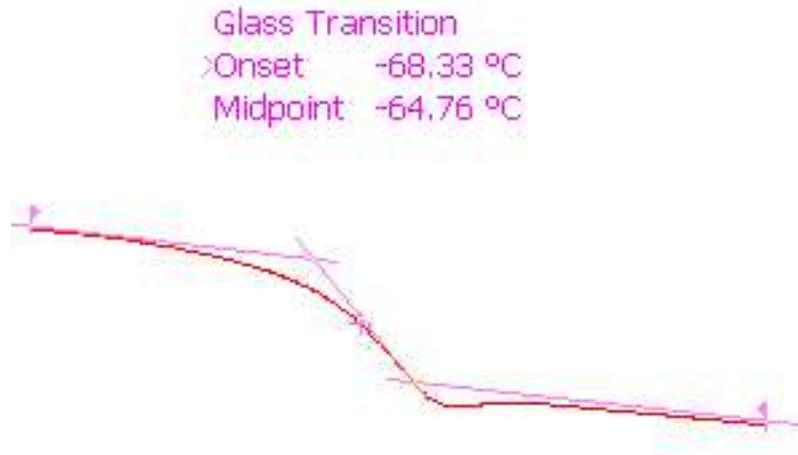
Figure 2.32: DSC Glass transition technique: BIIR
