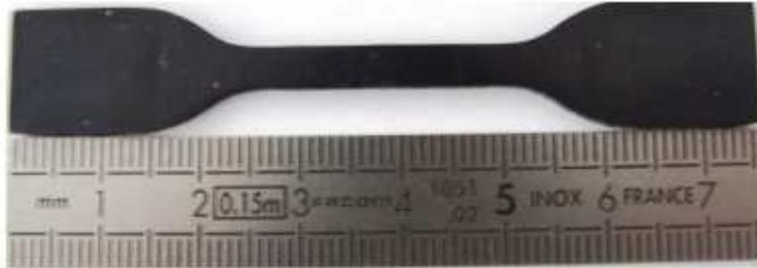
Figure 2.7: H2 Specimen (ISO 37 standard)
