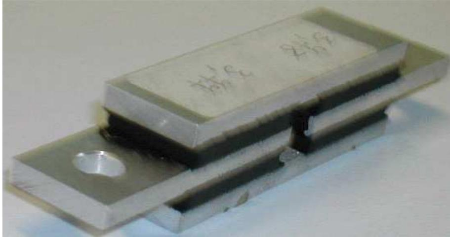
Figure 2.9: Quad-shear sample
