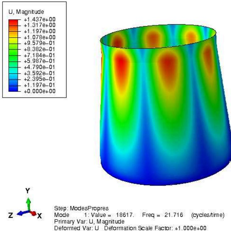
Figure 4.10: 1<sup>st</sup> fundamental lateral mode shape: Undamped Alu
