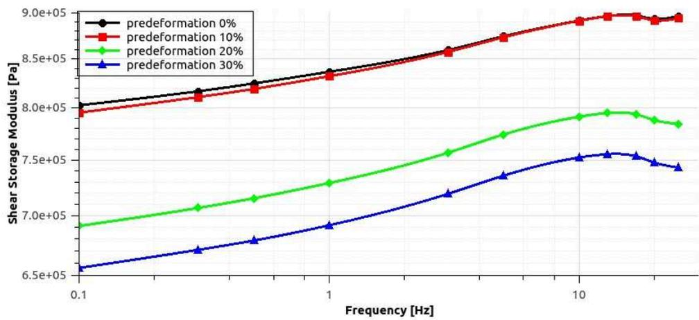
Figure 2.44: Shear modulus frequency and predeformation dependence: NR
