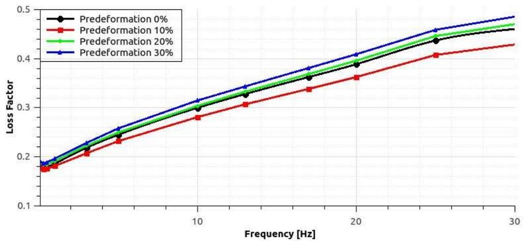
Figure 2.48: Loss factor frequency and predeformation dependence: NR/BIIR
