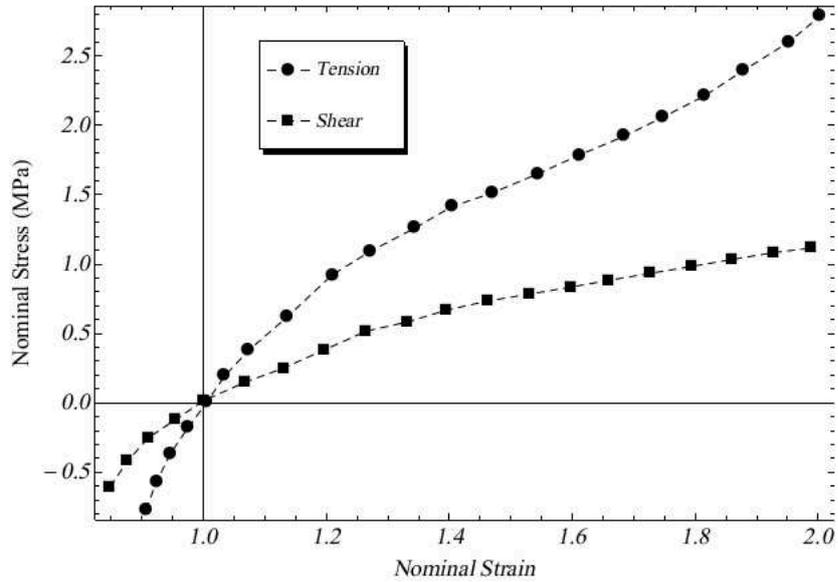
Figure 1.1: Nominal stress vs strain for quasi-static loadings [14]
