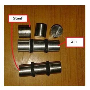
Figure 2.10: specimen preparation
