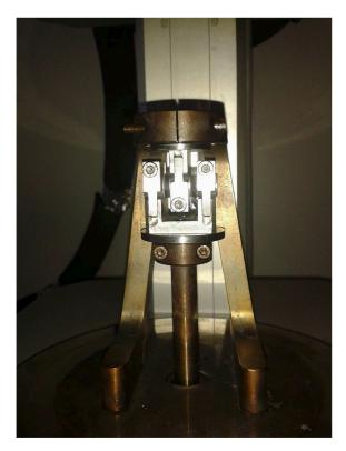
Figure 2.11: DMA shear specimen holder
