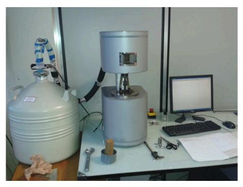
Figure 2.5: Metravib DMA 50N testing machine
