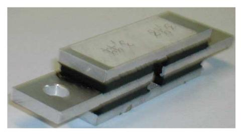
Figure 2.9: Quad-shear sample
