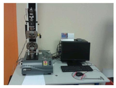
Figure 2.4: Instron 3345 testing machine
