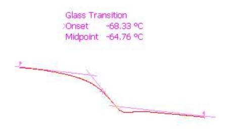
Figure 2.32: DSC Glass transition technique: BIIR
