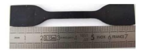
Figure 2.7: H2 Specimen (ISO 37 standard)
