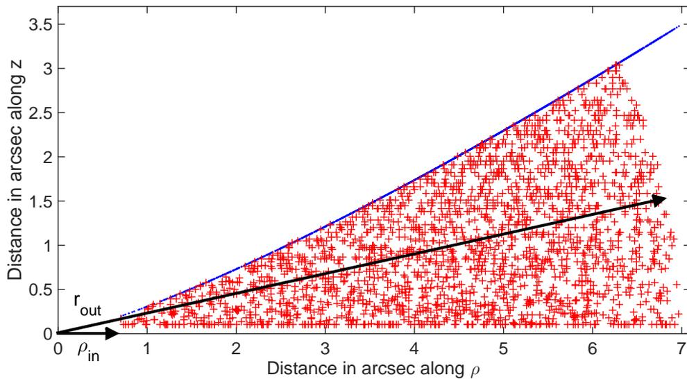
Figure 2.9 – Disk profile in cylindrical coordinates  $(\rho, z)$ . Grid points are shown in red whereas the specific pressure scale height  $h_0$  is plotted in blue. GASS automatically rejects any point above this height. The inner cylindrical and outer spherical radii ( $\rho_{in}$  and  $r_{out}$ ) can be identified as well.
