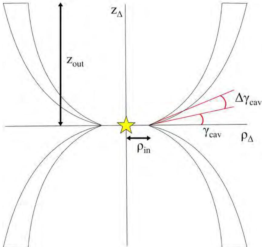
Figure 2.6 – Sketch showing the different parameters that define the structure of the outflow.  $\rho_{in}$  is the inner cylindrical radius of the outflow while  $z_{out}$  is the maximum height that the outflow can reach.  $\rho_{\Delta}$  and  $z_{\Delta}$  define the cylindrical axes of the outflow.  $\Delta\gamma_{cav}$  defines the width of the cavity walls.
