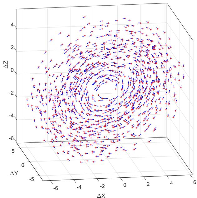
Fig. 7: Grid points distribution (red crosses) over the described model. The inner radius  $\rho_{in}$  is clearly visible as well as the two rotation angles  $\Theta$  and  $\Phi$ . The velocity vectors are plotted in blue and show the Keplerian rotation of the disk.
