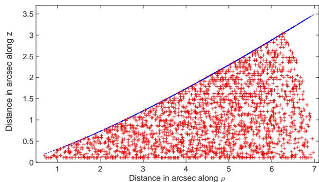
Fig. 8: Disk profile in cylindrical coordinates  $(\rho, z)$ . Grid points are shown in red whereas the specific pressure scale height  $h_0$  is plotted in blue. GASS automatically rejects any point above this height. The inner cylindrical and outer spherical radii ( $\rho_{in}$  and  $r_{out}$ ) can be identified as well.
