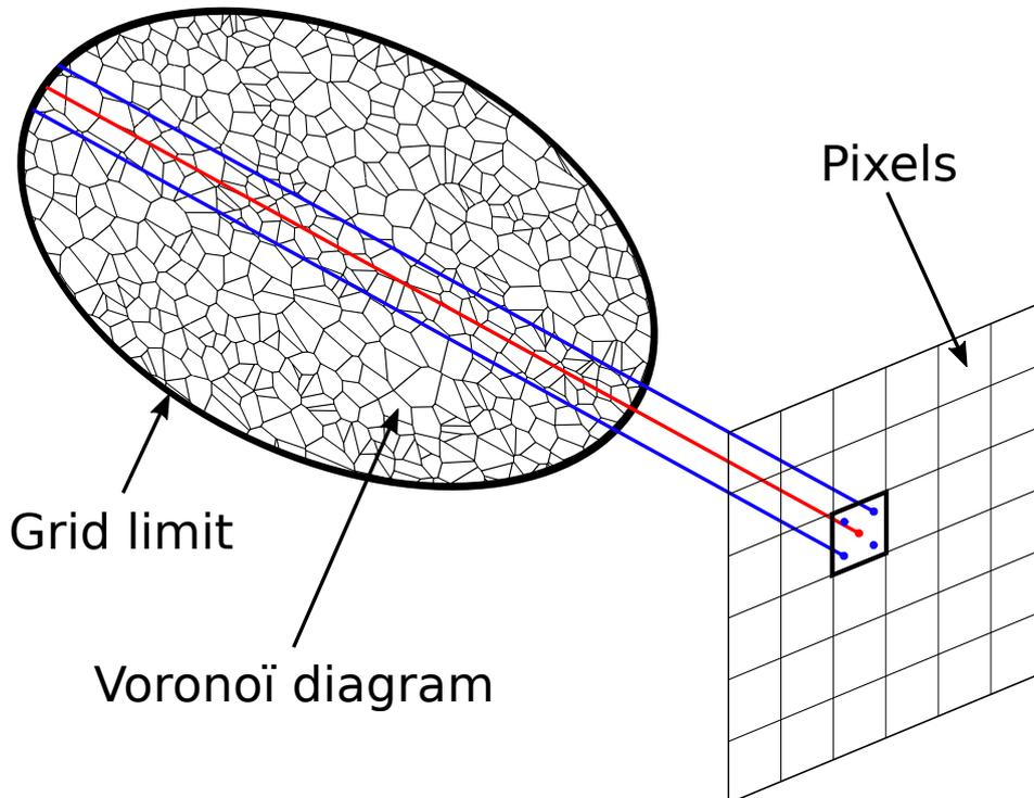
Figure 2.23 – Sketch explaining the *ray-tracing* of LIME. The pixel intensity is only determined with cells crossing the different line-of-sights. The red line is the line-of-sight located at the centre of a pixel, for *antialias* = 1. Blue ones shows the distribution of line-of-sights for *antialias* = 4.
