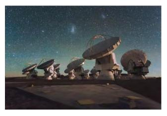
Figure 1.10 – The ALMA interferometer composed of 66 antennas, located on the Chajnantor plateau (Chile).
