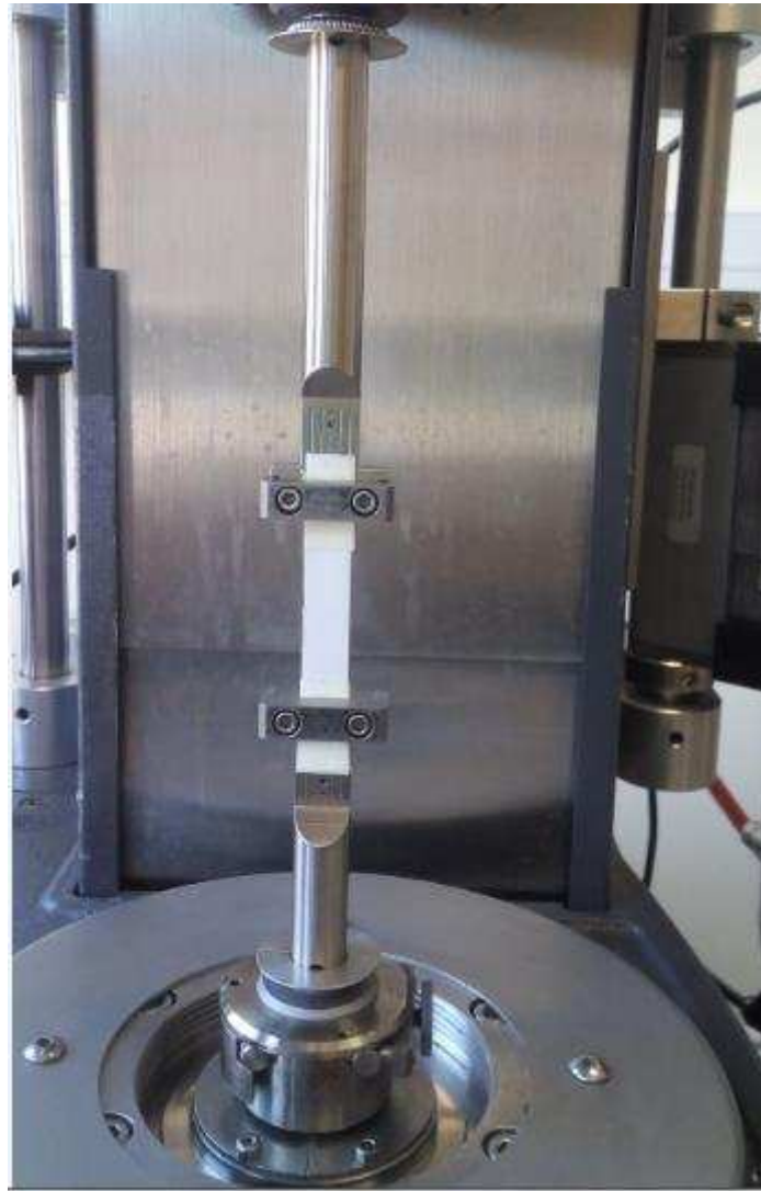
Figure II.8: Sample was prepared in the form of rectangular shape with dimensions of 30 x 10 mm from the electrospun fibrous membranes
