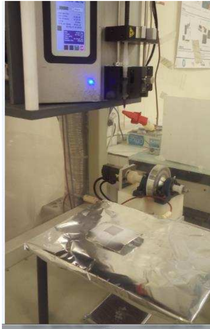
Figure II.5: Machine electrospinning with the static collector
