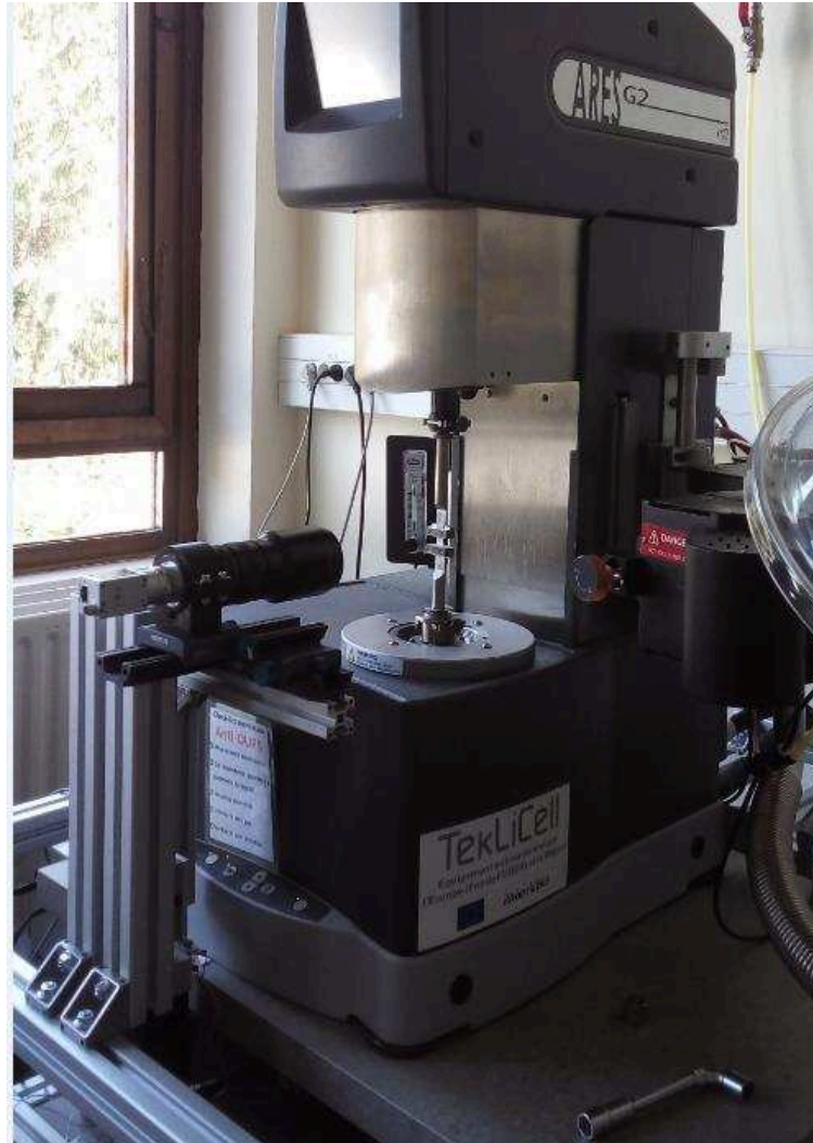
Figure II.7: Device for the mechanic (ARESG2) with camera
