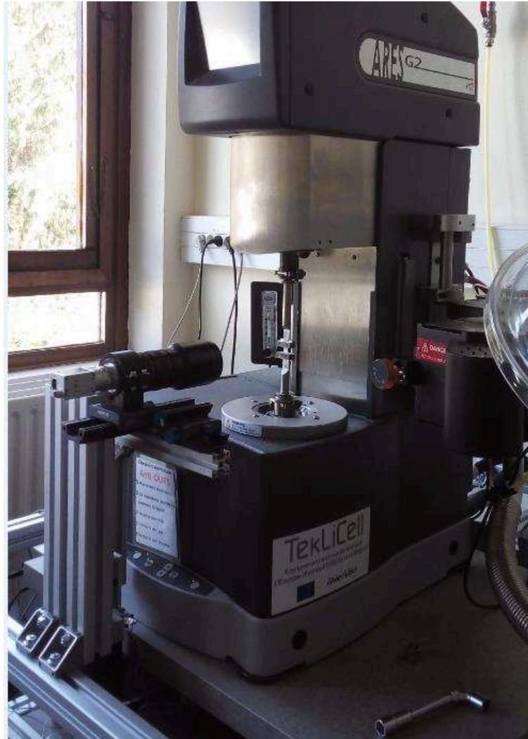
**Figure II.7: Device for the mechanic (ARESG2) with camera**
