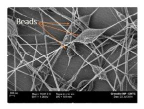
Figure I.5: SEM of poly (Ethylene Oxide) nanofibers Electrospum from aqueous solution  $2.9\% \, M_w$ :  $(1.0 \times 10^6) \, g/mol$
