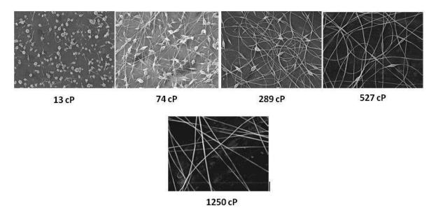
Figure I.7: Effect of solution viscosity on the fiber morphology<sup>(20)</sup>
