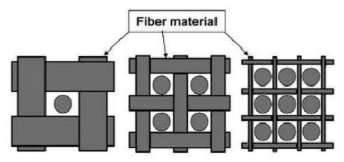
Figure I.18: Scheme of the relationship in principle between the diameter of the filaments and the filtered particles
