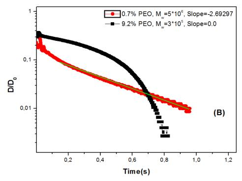
Figure III.1.18. B: Normalized filament diameter in CaBER experiments for PEO solutions. The time t=0 is defined as the time at which the upper plate has reached its final position. Mw ~  $3.0\times10^5$  and  $5.0\times10^6$  g/mol, C=0.7 wt% and 9.2 wt %. ( Diameter as a function of time (log/linear)
