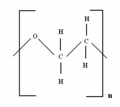
Figure II.1: Chemical structure of PEO
