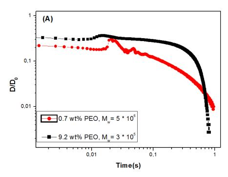
Figure III.1.18.A: Normalized filament diameter in CaBER experiments for PEO solutions. The time t=0 is defined as the time at which theupper plate has reached its final position. Mw ~  $3.0 \times 10^5$  and  $5.0 \times 10^6$  g/mol, C = 9.2 wt% and 0.7 wt %.( Diameter as a function of time (Log/Log)
