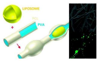
Figure 1.20: Schematic representation of the PVA/PCL core/shell fibers loaded with liposome and their SEM and confocal microscopy images<sup>(122)</sup>
