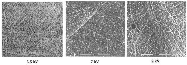
Figure I.10: Bead formation at higher voltage<sup>(76)</sup>
