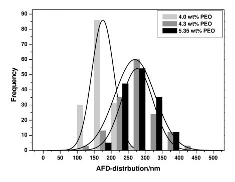
Figure III.1.15: The average of diameter distribution of 4.0 wt%, 4.3 wt% and 5.35 wt% of PEO  $\sim 1.0 \times 10^6 \rm g/mol$
