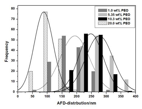
Figure III.1.16: The average of diameter distribution of 20.0 wt%, 10.3 wt%, 5.35 wt%, and 1.0 wt% of PEO ~  $1.0 \times 10^5$ ,  $3.0 \times 10^5$ ,  $1.0 \times 10^6$ , and  $5.0 \times 10^6$  g/mol respectively
