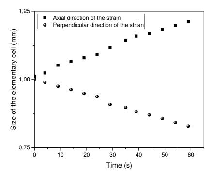
Figure III.2.7: Evolution of the size of the elementary cell in the axial and perpendicular directions of the strain for the structured membrane.
