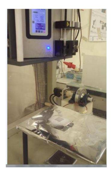
Figure II.5: Machine electrospinning with the static collector
