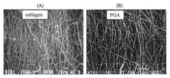
Figure I.14: Aligned nanowires collagen and PGA
