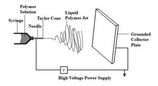
Figure I.4: General Electrospinning schematic
