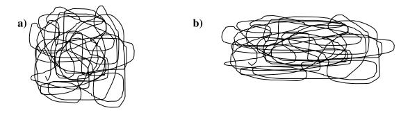
Figure III.2.9: Sketch of the random network a) at rest and b) under stretching
