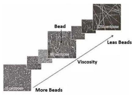
Figure I.8: SEM images of electrospun nanofibers with beads from different polymer concentration solutions<sup>(20)</sup>
