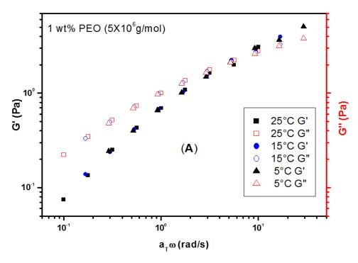
Figure III.1.8A: Storage modulus G' and loss modulus G'' as a function of angular frequency for 1.0 wt % (5.0 × 10<sup>6</sup> g/mol) polymer solution PEO at different temperature
