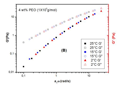
Figure III.1.8B: Storage modulus G 'and loss modulus G"as a function of angular frequency for 4.0 wt%  $(1.0 \times 10^6 \text{g/mol})$
