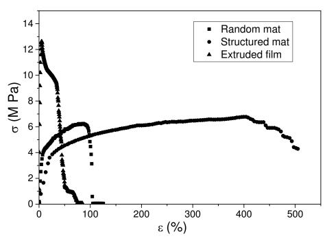
Figure III.2.5: Curve stress-deformation of extuded film, electrospun membranes having a random orientation of fibers and a square like structure. Stretch velocity of 0.25 mm/s
