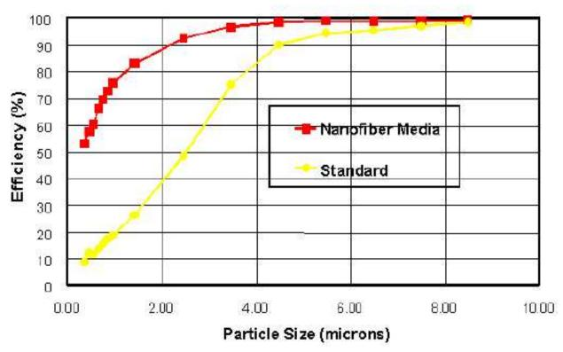
Figure 1.19: Fractional efficiency (Filtration Efficiency versus particle size) for a standard cellulose media and nanofiber filter media (119)
