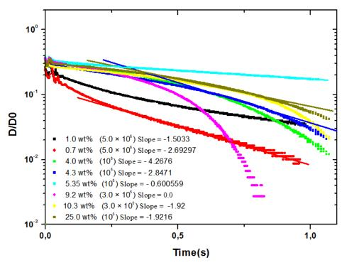
Figure III.1.17: Normalized filament diameter in CaBER experiments for PEO solutions. The time t=0 is defined as the time at which theupper plate has reached its final position.  $Mw \sim 10^5, 3.0 \times 10^5, 10^6 \text{ and } 5.0 \times 10^6 \text{ g/mol and}$
