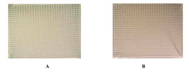
Figure III.2.3: The membranes produced by using the microstructure collector: A) represent 4.0 wt% PEO  $(1.0 \times 10^6)$  and B) 10.3 wt% PEO  $(3.0 \times 10^5)$
