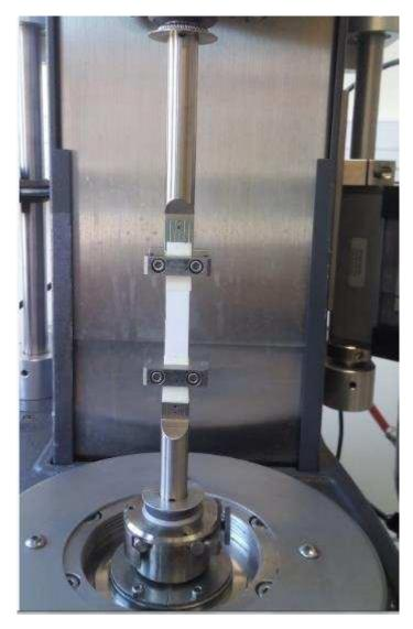
Figure II.8: Sample was prepared in the form of rectangular shape with dimensions of 30 x 10 mm from the electrospun fibrous membranes
