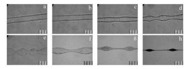
Figure I.9: Onset of axisymmetric instability causing bead formation in the fibers. The pictures taken at different distances from the needle. a. 1 cm, b. 3cm, c. 5cm, d. 7cm, e. 9cm,f. 12cm, g. 15cm, h. 30 cm
