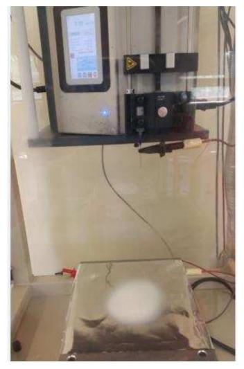
Figure II.4: Machine electrospinning with the aluminum foil collector
