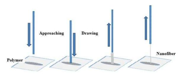
Figure I.2: Drawing process
