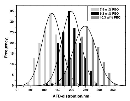
Figure III.1.14: The average of diameter distribution of 7.5 wt%, 9.2 wt% and 10.3 wt% of PEO ~  $3.0 \times 10^5 \text{g/mol}$
