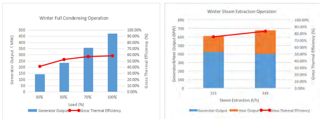
Fig. 3.6 Performance of winter full condensing/ steam extraction operating condition
