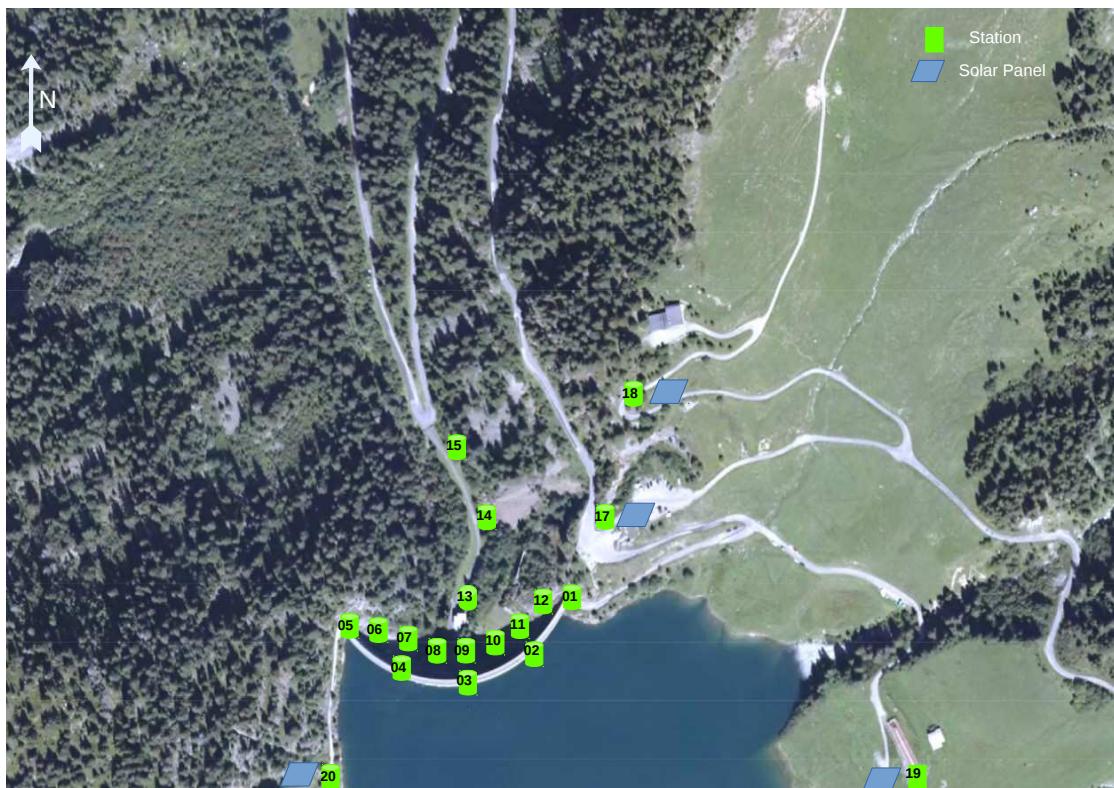
FIGURE 2.7: Position of seismological stations on and around the dam of Saint Guérin.
