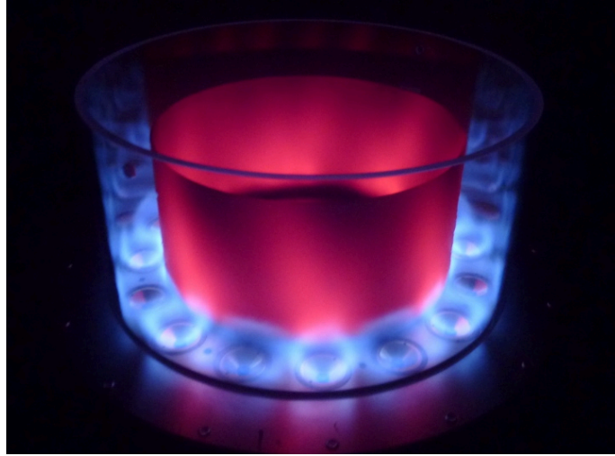
Figure 6.11. Visualization of the thermal effects. 90° cup. U_b \approx 17.1 \text{ m.s}^{-1} .
