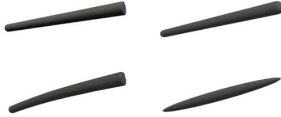
Figure E-1 Shapes of fibres used in our computations: (a) straight cylindrical fibre; (b) cylindrical fibre with rounded ends; (c) curved cylindrical fibre (curvature radius is around 25 mm); (d) ellipsoidal fibre.
