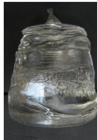
90 kg sapphire crystal grown by F.J.Bruni using Kyropoulos method [17]
