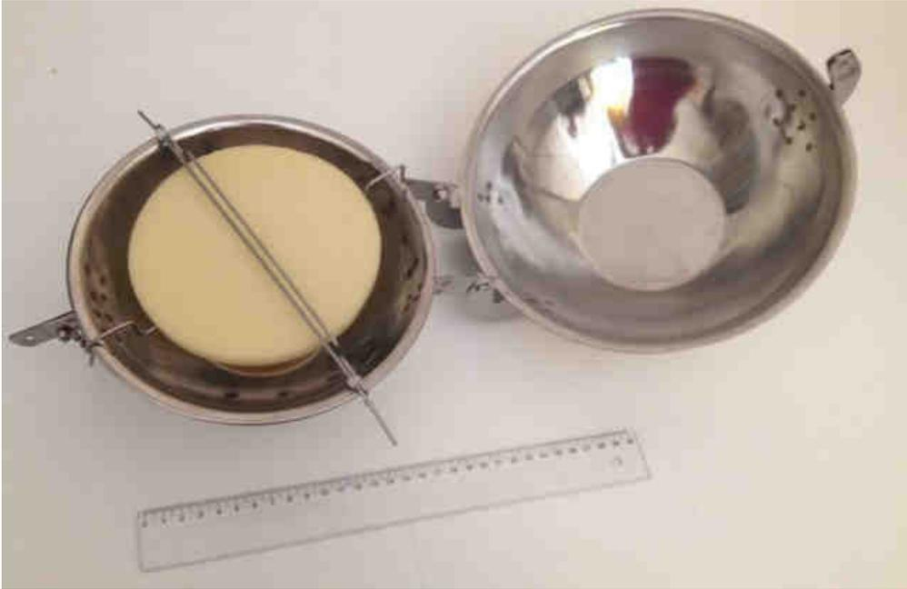
Figure 1-2 – Placement of a PUF disk inside its housing
