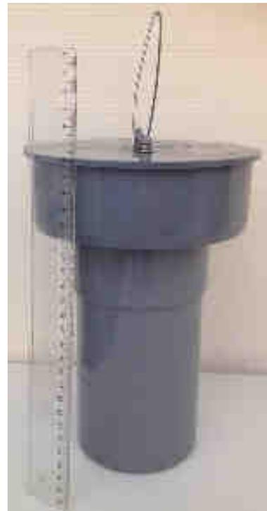
**Figure 1-5 – PVC housing for the XAD®-2 tube**
