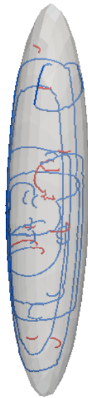
Figure 5.18 – Dislocation microstructure at step 1070 in Cigar grain
