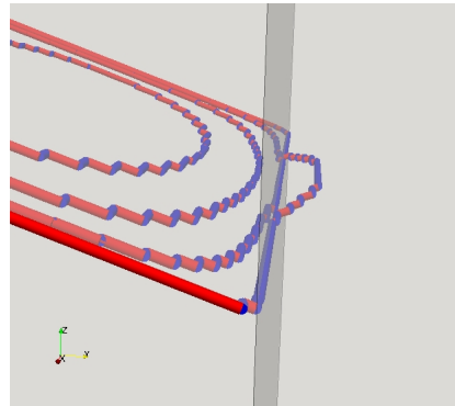
Figure 4.26 – Slip transmission across CTB at step \mathbf{P}+T_2
