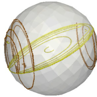
Figure 5.6 – Dislocation activity with cross slip in Sphere
