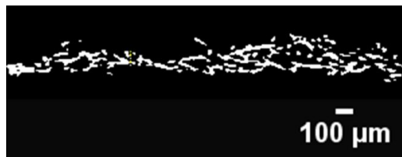
Figure 1-8 : Cross section of a low grammage paper ( 23 \text{ g m}^{-2} ) presented in the X-ray binarised image (fibres in white). Significant local thickness variation can be observed.
