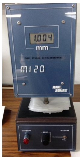
Figure 2-5 : Apparatus to measure thickness of paper installed in LGP2, Grenoble.
