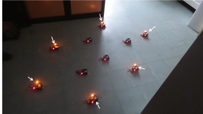
Figure 3.10: Execution of D-LPCN using real Arduino/XBee sensor nodes.
