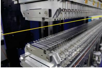
Figure 3.15: The jaws of undulators are made up of small magnets producing alternating magnetic fields. The magnetic fields make the electron bunches move along wavy trajectories of period  $\lambda_u$  and angular deviation  $\alpha$ . The magnetic field intensity can be adjusted by varying the gap between the jaws.
