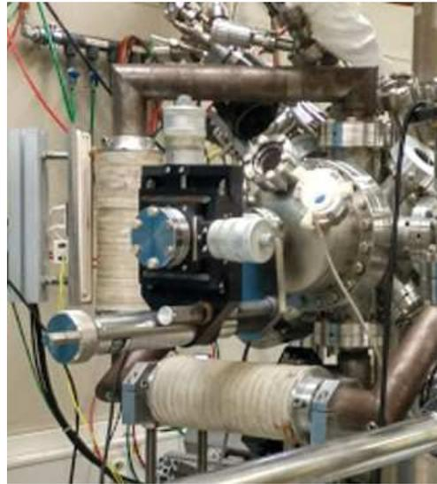
Figure 3.10: The experimental apparatus used for MOKE measurements at ID03. The electromagnets are mounted on the flanges of the UHV chamber in which the sample is placed.
