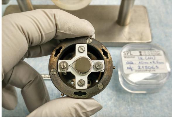
Figure 3.25: Sample mounted on the sample-holder. Two screws are fixing a Tantalum wire holding the sample in place. Alternatively, a Ta clip can be used instead of the wire.
