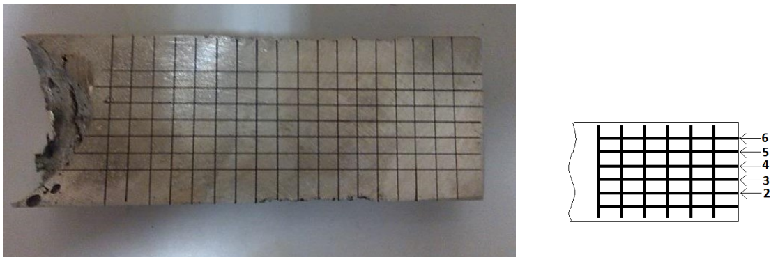
Fig 48 Sample of magnesium alloy EK21 subjected to hardness test
