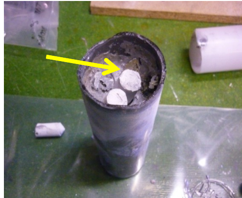
Fig 72 Pure aluminium with agglomerates of Al 2 O 3 particles
