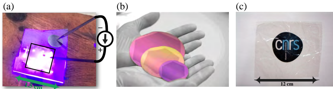
Figure 0.8: Graphene for device applications. (a) Photo of a working GaN quantum well LED with graphene electrode. (b) Graphene transferred on 2, 3 and 4 inches Si/SiO 2 wafer. (c) Centimeter scale polymer-graphene transparent membrane.
