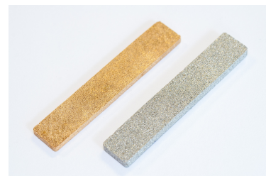
(c) Preformed slabs of partially-sintered bronze and stainless steel powders (5 cm in length)
