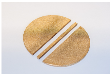
(a) EDM cut of a partially-sintered bronze bar (7 cm in length)
