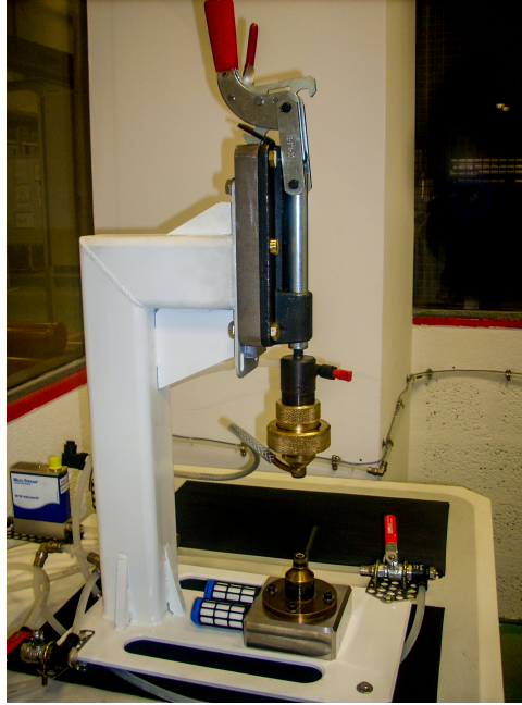
Figure 4.6: Permeability bench used by the company Sintertech .
