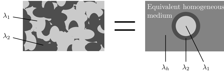
Figure 3.2: Principle of the asymmetric model of Bruggeman (1935). The grains of the phase 1 are surrounded by the phase 2 which is included in a mean phase having an intermediate composition which has the effective property of the two-phase material
