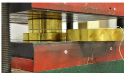
**Figure 31.** Experimental set-up for calibration of the circular mold.
