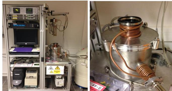
**Figure 61.** Towards the left is the experimental set-up of dielectric spectroscopy and towards the right is the Cryostat.
