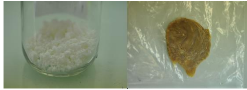
Figure 33. To the left is the image of surfactant-modified MFC and to the right is the blend of PLA-MFC obtained from internal mixer.
