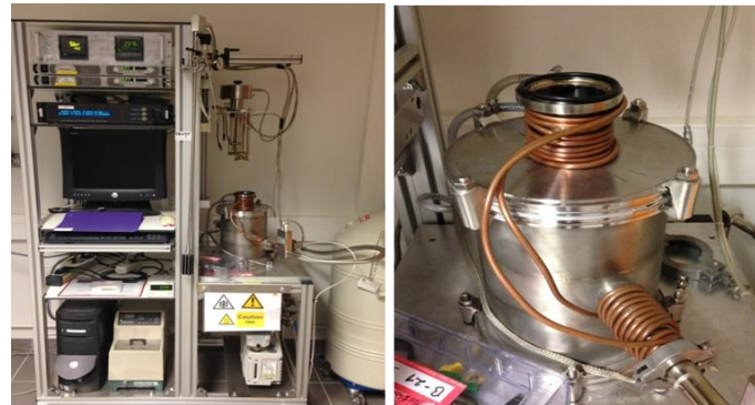
Figure 61. Towards the left is the experimental set-up of dielectric spectroscopy and towards the right is the Cryostat.
