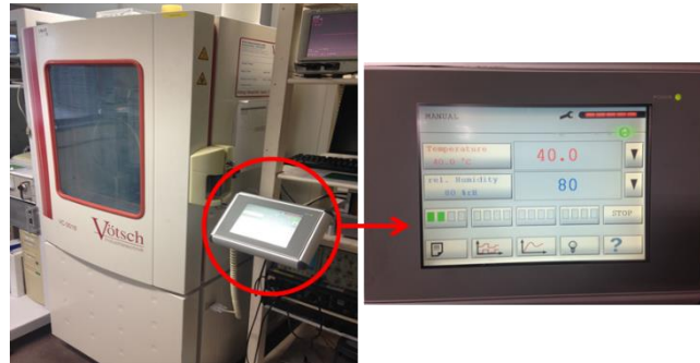
Figure 47. Towards the left is the Vötsch climatic test chamber and towards the right is the enlarged image of the display (touch) screen.
