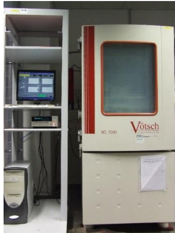
Figure 120. Experimental set-up showing the climatic test chamber with Model 8009 Resistivity Chamber (not seen) inside it.
