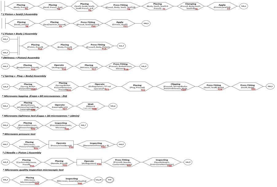
Annex C – Figure 1: The assembly generic process model
