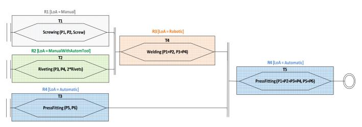
Figure 7: An example of using tasks vocabulary to represent an automation alternative
