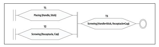
Figure 9: The initial assembly tasks generic representation for the given example
