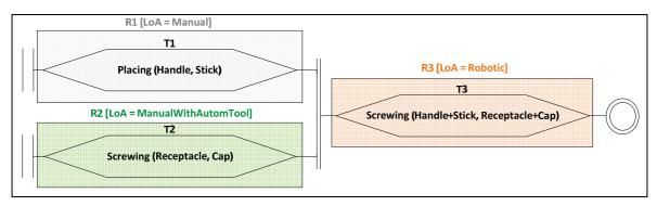
Figure 10: An automation alternative representation for the given example
