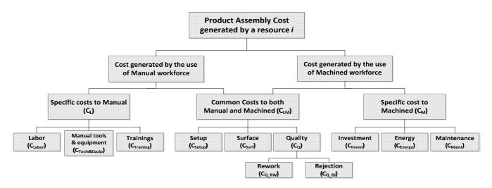
Figure 21: The assembly cost generated by a process resource according to its LoA: the cost model architecture
