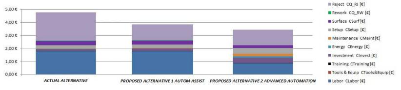
Annex D Figure 1: Obtained assembly costs per product for the different assembly systems alternatives
