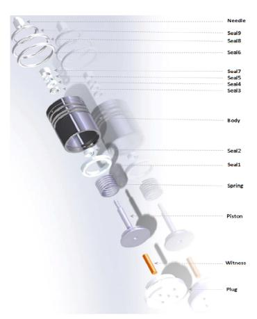
Figure 24: The product components to be assembled
