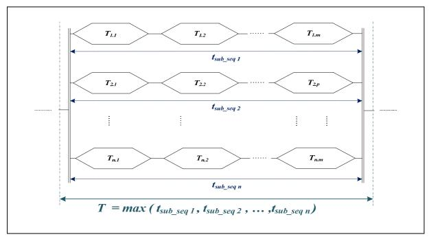
Figure 14: Time estimation for parallel sub-sequences of tasks
