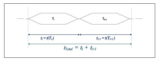
Figure 13: Time estimation for serial tasks
