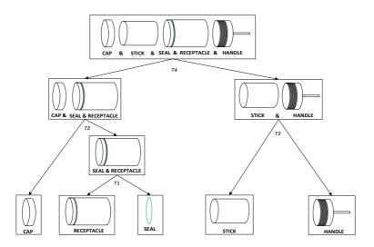
Figure 28: The defined assembly sequence
