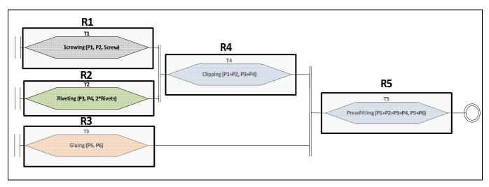
Figure 18: An alternative of resources assignments to tasks
