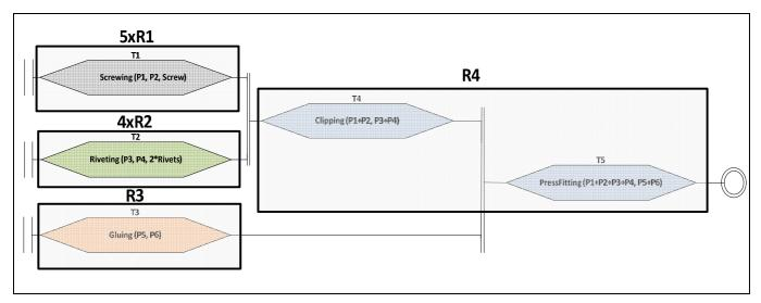
Figure 19: A configuration of automation option for a balanced process
