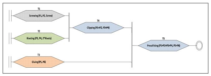
Figure 17: An automation combination to process tasks for a product assembly example
