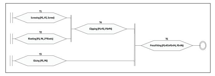
Figure 16: A product assembly example shown by its ASML tasks representation
