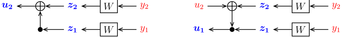
Figure B.1 – The decoding algorithm over the two synthetic channels (left) W^- : \mathbb{F}_2 \rightarrow \mathcal{Y} \times \mathcal{Y} , (right) W^+ : \mathbb{F}_2 \rightarrow \mathcal{Y} \times \mathcal{Y} \times \mathbb{F}_2
