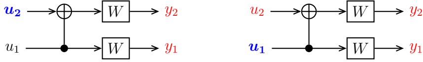
Figure 3.3 – The two synthetic channels (left) W^- : \mathbb{F}_2 \rightarrow \mathcal{Y} \times \mathcal{Y} , (right) W^+ : \mathbb{F}_2 \rightarrow \mathcal{Y} \times \mathcal{Y} \times \mathbb{F}_2
