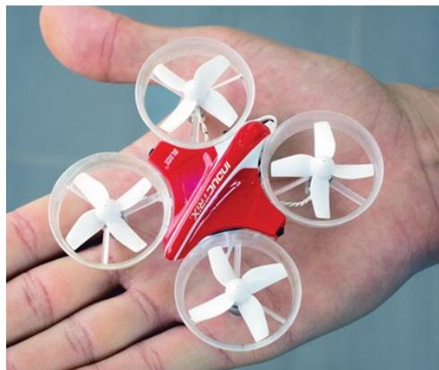
Figure 5.7: Inductrix quadcopter.
