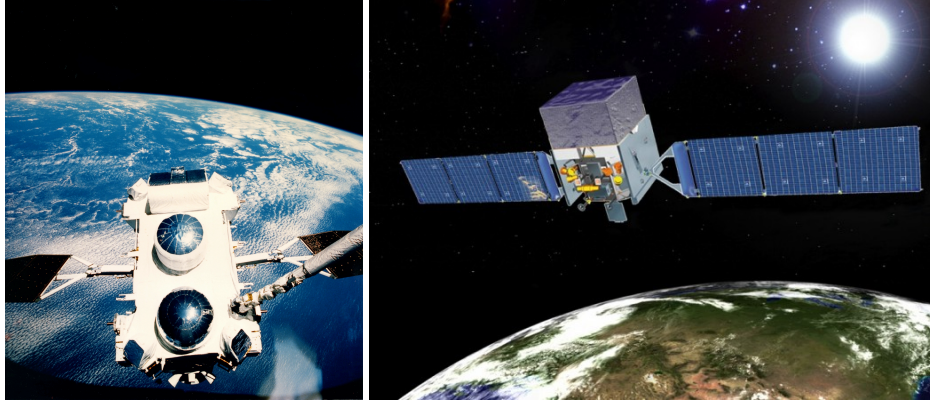
FIGURE 1.8: Left: Deployment of the CGRO where EGRET can be seen (the dark bump at the bottom) along with OSSE and COMPTEL. Right: Illustration of the Fermi satellite with the LAT mounted on top.
