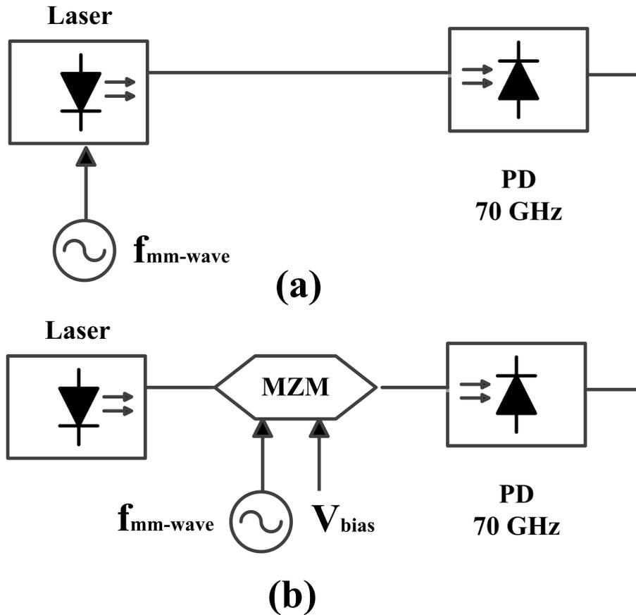
Figure 1.7: Generation of mm-wave using (a) Direct (b) External modulation.
