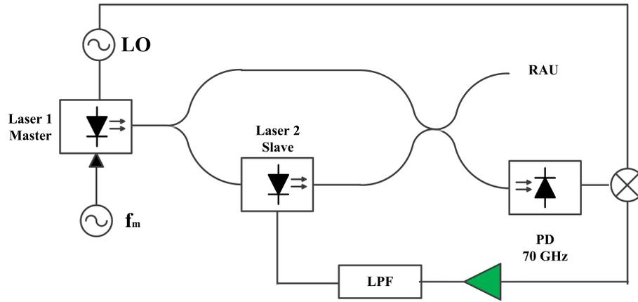
Figure 1.6: Generation of mm-wave using OPLL and OIL.
