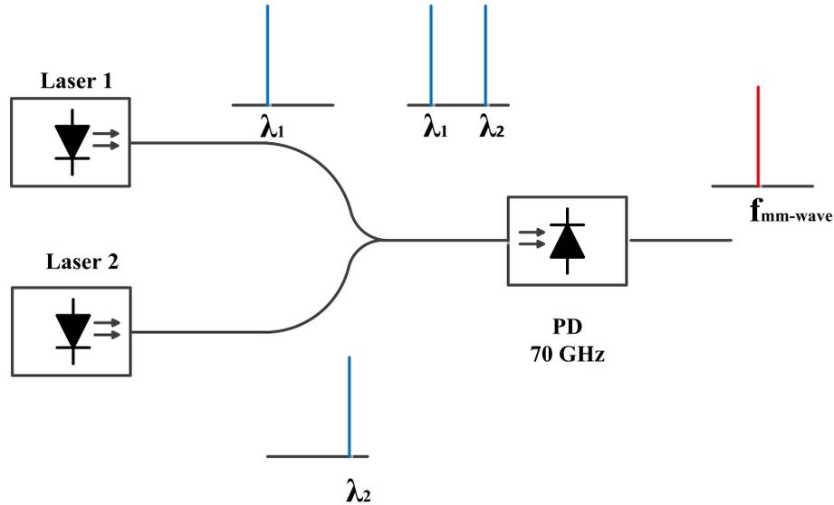
Figure 1.3: Two free running lasers generating mm-wave.
