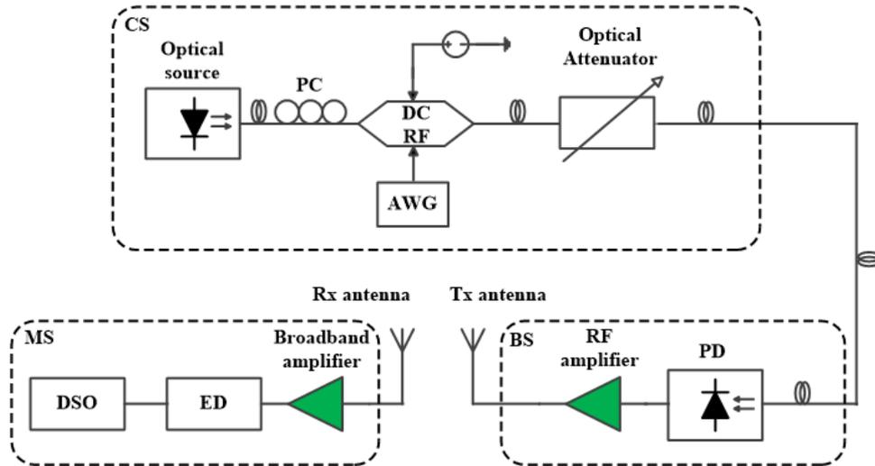
Figure 2.9: Experimental setup for 60 GHz RoF wireless system based on two independent lasers or PMLLD.
