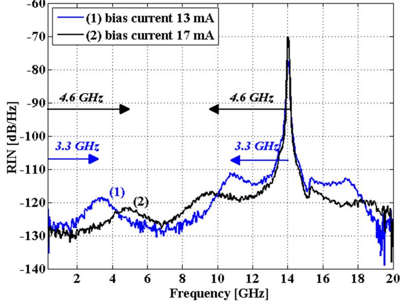
Figure 2.4: RIN of the beat note at 14 GHz for two different bias currents of the first laser DFB<sub>1</sub>.
