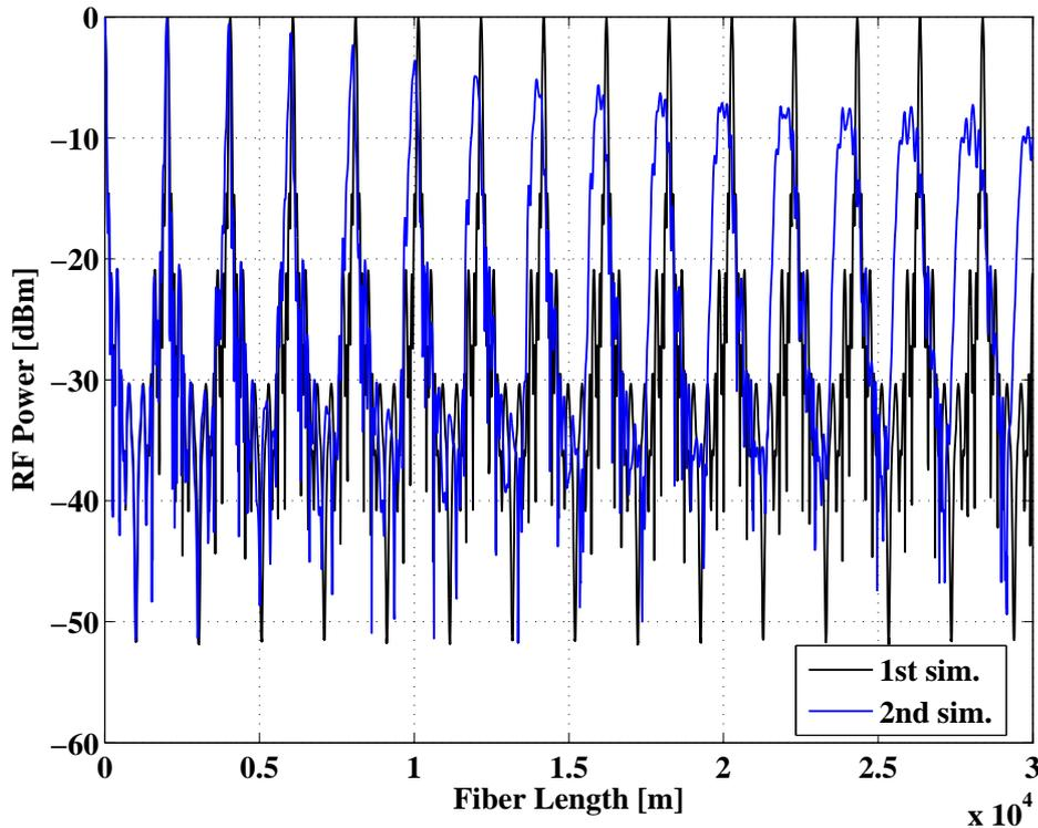
Figure 4.2: Simulation of chromatic dispersion on a 60 GHz RoF communication network for different values of GVD.
