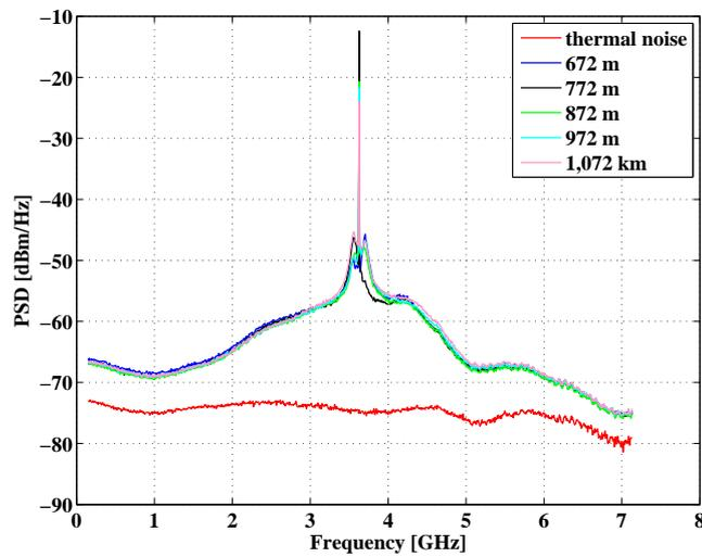
Figure 4.7: Electrical spectra of mode partition noise on a 60 GHz RoF communication system for different fiber lengths.
