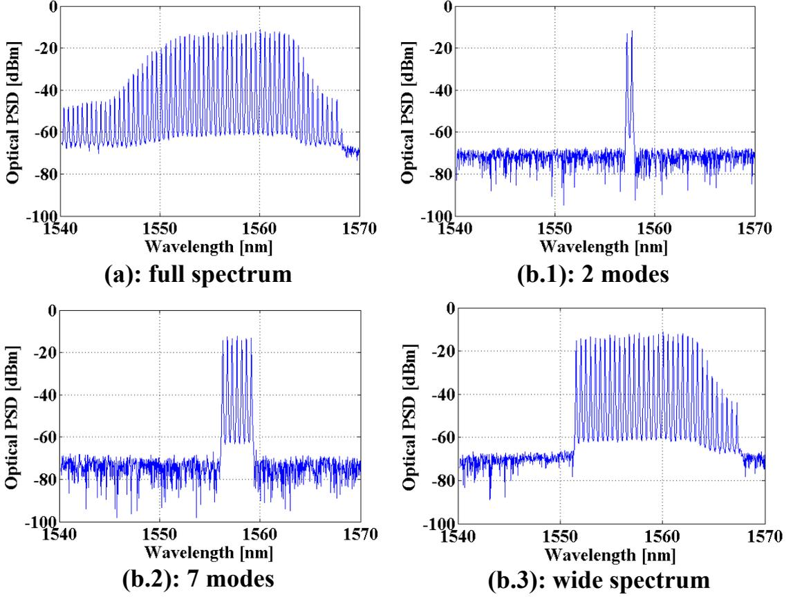
Figure 3.2: Optical spectrum of PMLLD for different bandwidth of WSS at biased current 209 mA.
