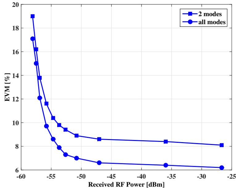
Figure 3.10: Measured EVM as a function of received RF power for filtered two optical modes and entire optical spectrum at 100 Mbps of QPSK modulation.
