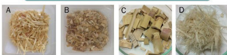
Figure 1. Dried material before mercerization, bleaching, and hydrolysis. A) maize husk, B) bean shell, C) Bagasse bark, and D) Bagasse core
