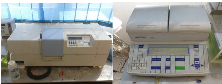
Figure 2: Photography of the polarimeter (left) and the refractometer (right) used in this work.
