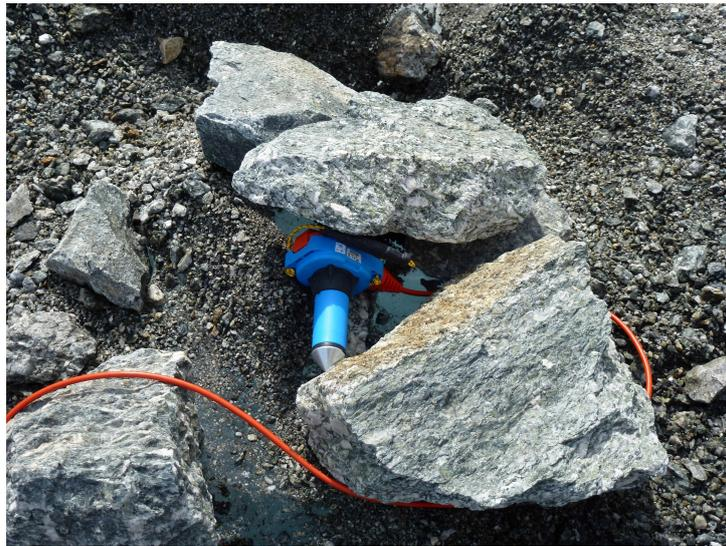
Figure 9.7.: Pictures of the geophone used for our experiment
