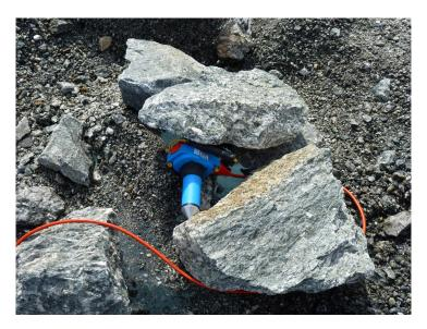
Figure 9.7.: Pictures of the geophone used for our experiment
