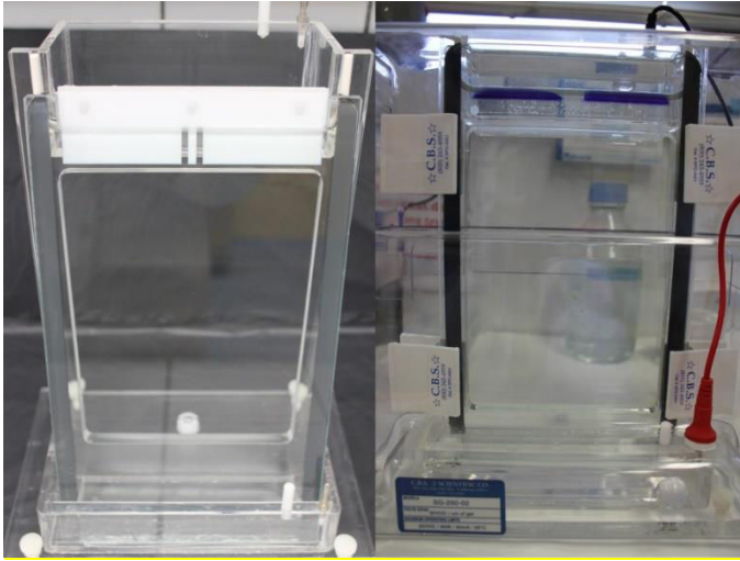
Figure 9: 5% acrylamide gel assembly
