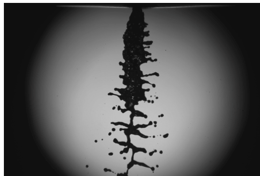
Figure 3.3: Production and disintegration of a water sheet (Injection pressure \Delta P_i = 0.1 \text{ MPa} )
