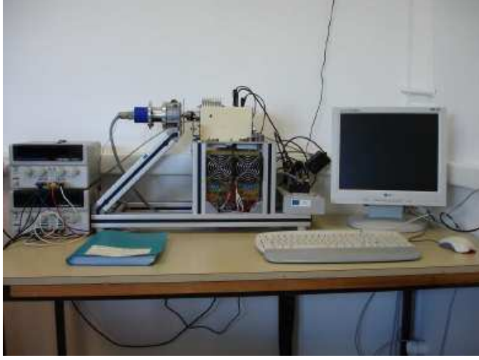
Figure 6.2: PMSM test-bench located at Centrale Lille.
