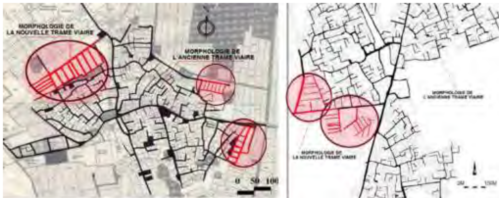
Figure 4.25. Morphological transformation of village structures during the urbanisation process [Source: Tran Nhat Kien, 2010]
