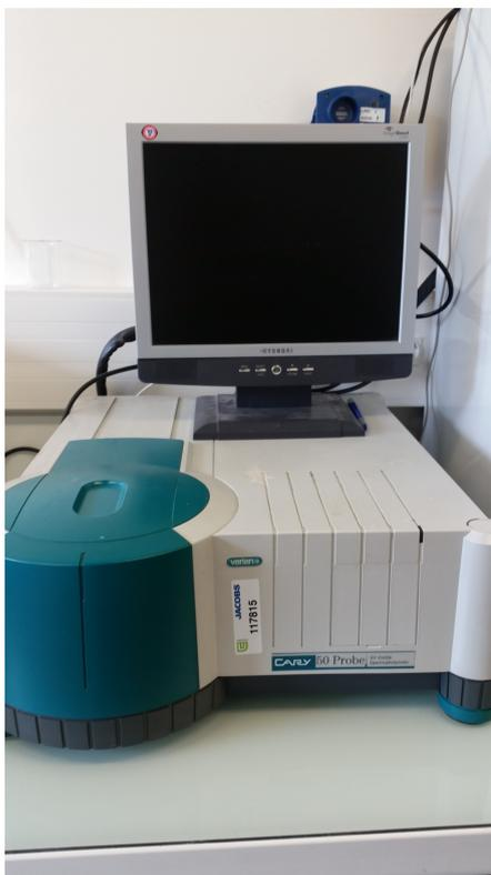
FIGURE D.4: The UV-visible spectrophotometer.
