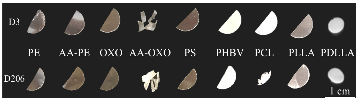
Figure 1: Physical evolution of the nine polymer pieces after 3 and 206 immersion days in seawater.
