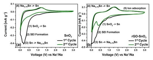
**Figure 4.8** Cyclic voltammogram (CV) of (a) SnO<sub>2</sub> and (b) rGO-SnO<sub>2</sub> in NIB at a scan rate of 0.1 mV s<sup>-1</sup>
