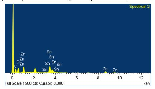
Figure 6.3 Energy dispersive X-ray mapping of ZnSnO<sub>3</sub> hollow cubes.
