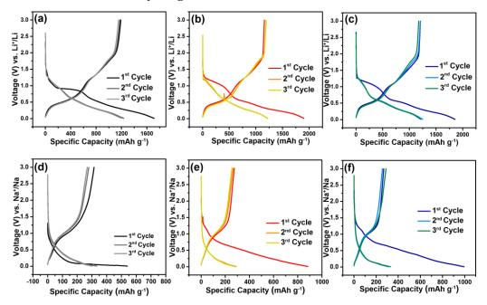
**Figure 5.8** Galvanostatic discharge curves of pristine  $SnO_2$ ,  $SnO_2+N3\%$  and  $SnO_2+N8\%$  in (a-c) LIB and (d-f) NIB.
