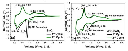
**Figure 4.7** Cyclic voltamogram (CV) of (a)  $SnO_2$  and (b)  $rGO-SnO_2$  in LIB at a scan rate of 0.1 mV s<sup>-1</sup>
