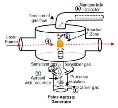
Figure 3.1 Schematic of the laser pyrolysis working procedure
