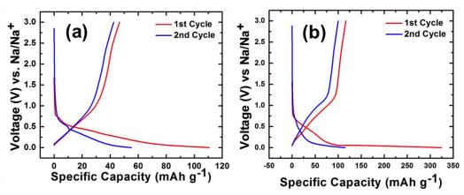
**Figure 6.6** Initial galvanostatic charge-discharge curves of (a) ZnO and (b) ZnO-SnO<sub>2</sub> in NIB at 30 mA g<sup>-1</sup>.
