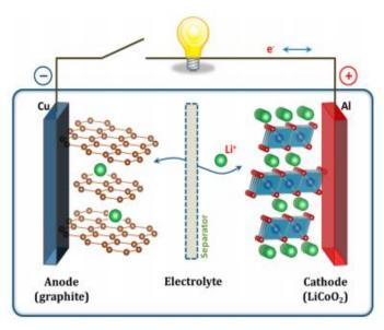
Figure 2.1 Operational illustration of the Li-ion battery<sup>2</sup>
