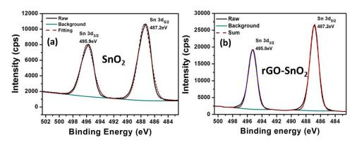
**Figure 4.6** Binding energy values of Sn 3d measured from X-ray photoelectron spectroscopy (XPS) for (a) pristine SnO<sub>2</sub> and (b) rGO-SnO<sub>2</sub>.
