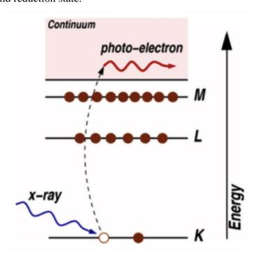
**Figure 3.5** Photoelectric effect, in which X-ray is absorbed and a core-level electron is ejected out from the atom
