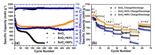
**Figure 5.9** (a) Cycling performance and the corresponding Columbic efficiency (C.E) at 1.4 A g<sup>-1</sup>. (b) Rate performance (discharge (solid) and charge (hollow)) of pristine SnO<sub>2</sub> vs. N-doped SnO<sub>2</sub> within a voltage window between 0.01 – 3.00 V vs. Li<sup>+</sup>/Li.
