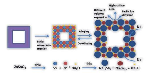
**Figure 6.10** Schematic describing the energy storage process in polycrystalline  $ZnSnO_3$  hollow cubes. The  $ZnSnO_3$  first undergoes an irreversible conversion process into metallic Zn and Sn and subsequently, a reversible alloying process ensues, producing  $Na_{15}Sn_4$  and  $NaZn_{13}$  alloys.
