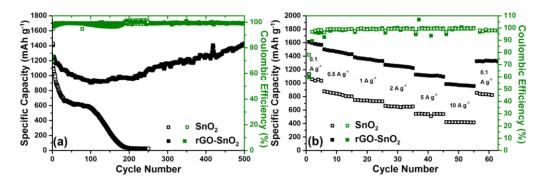
**Figure 4.11** (a) Lithiation cycling performance of rGO-SnO<sub>2</sub> and pristine SnO<sub>2</sub> at 2 A g<sup>-1</sup> and 1.4 A g<sup>-1</sup> respectively. (b) Lithiation rate performance of rGO-SnO<sub>2</sub> and pristine SnO<sub>2</sub> at various current densities.
