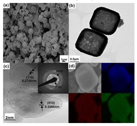
**Figure 6.2** (a) low magnification SEM image of the as-synthesized ZSO-H (b) TEM image of polycrystalline hollow cubes (c) HRTEM revealing lattice spacing and the agglomerate of nanoparticles (inset shows typical polycrystalline Selected Area Electron Diffraction (SAED) pattern) (d) SEM-EDX element mapping of Zn, Sn and O on a single cube.
