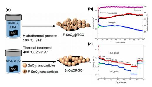
**Figure 2.6** (a) Schematic of hydrothermal synthesis of F-doped SnO<sub>2</sub> and F-doped SnO<sub>2</sub>@graphene. Comparison of (b) cycling performance at 0.1 A g<sup>-1</sup>and (c)rate capabilities
