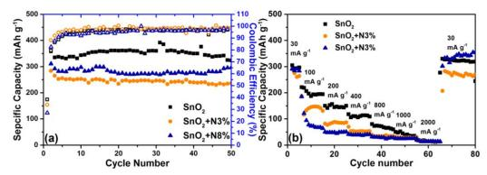
**Figure 5.10** (a) Cycling performance and the corresponding Columbic efficiency (C.E) at 30 A g<sup>-1</sup>. (b) Rate performance (discharge (solid) and charge (hollow)) of pristine  $SnO_2$  vs. N-doped  $SnO_2$  within a voltage window between 0.01 - 3.00 V vs.  $Na^+/Li$ .
