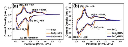
**Figure 5.6** (a)  $1^{st}$  and (b)  $2^{nd}$  lithiation cycle CV curves for the laser pyrolysed samples at 0.1 mV s<sup>-1</sup>. The sharp peak at ~0.8 V corresponds formation of SEI layer on the surface of the electrode during the initial discharge process.
