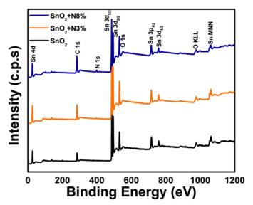
**Figure 5.3** General XPS plot comparing pristine SnO<sub>2</sub> vs. N-doped SnO<sub>2</sub>. The peaks are calibrated with respect to C 1s standard peak at 284.8 eV.
