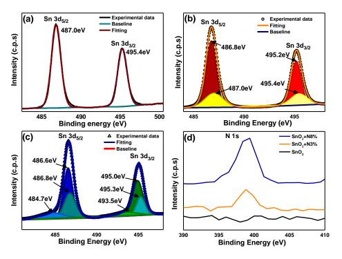
**Figure 5.4** Sn 3d XPS peaks of (a) pristine SnO<sub>2</sub>, (b) SnO<sub>2</sub>+N3%, and (c) SnO<sub>2</sub>+N8%. (d) is the N 1s XPS peak which displays relatively higher peak intensity with increasing NH<sub>3</sub> content. Additional shoulder peak at 484.7 and 493.4 eV in (c) reveals
