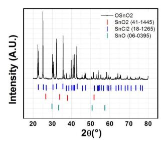
**Figure 4.1** XRD pattern after using  $SnCl_4$  as a precursor for laser pyrolysis in air (5.5 slm) and  $C_2H_4$  (0.3 slm). OSnO2 corresponds to the product and compared to JCPDS standards of tetragonal  $SnO_2$ ,  $SnCl_2 \cdot 2H_2O$  and SnO.
