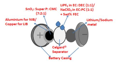
**Figure 3.7** A schematic of the coin cell and its components for both Li and Na ion battery.
