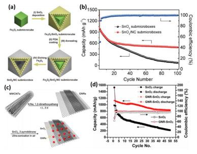
**Figure 2.5** (a) Schematic on the template-etching method for preparation of N-doped carbon coated SnO<sub>2</sub> (b) and its corresponding cycling performance.<sup>63</sup> (c) Preparation methodology for obtaining SnO<sub>2</sub> anchored on graphene nanoribbons. (d) Comparison between electrochemical properties of pristine SnO<sub>2</sub> and graphene nanoribbon-SnO<sub>2</sub><sup>77</sup>
