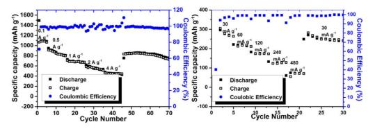
Figure 6.9 Rate performances of ZnSnO<sub>3</sub> hollow cubes in (a) LIB and (b) NIB
