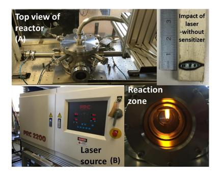
**Figure 3.3** In a clockwise direction from top left-hand corner, (A) illustrates the birdeye view of the reactor chamber as labeled in Figure 3.2. Beside it is the impact of the laser with wooden plank without the presence of sensitizer gas. Bottom right depicts the reaction zone in the presence of  $C_2H_4$  as sensitizer and air as a carrier gas. The last picture (B) corresponds to the  $CO_2$  laser source utilized during laser pyrolysis.
