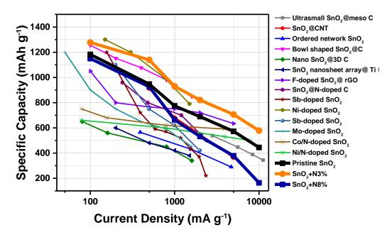
**Appendix A3.** Capacity vs. current density comparison between laser pyrolyzed samples (highlighted) and recently reported  $SnO_2$  materials. The references selected are based on 2 categories:  $SnO_2$ -carbon containing composites and element doped  $SnO_2$  compounds. Laser pyrolyzed  $SnO_2 + 3\%N$  shows the best performance at both low and high current densities, even without the presence of conductive carbon. Capacities plotted are average obtained from the rate performance- results.
