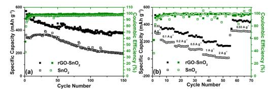
**Figure 4.12** (a) Sodiation cycling performance of rGO-SnO<sub>2</sub> and pristine SnO<sub>2</sub> at 30 mA g<sup>-1</sup>. (b) Sodiation rate performance of rGO-SnO<sub>2</sub> and pristine SnO<sub>2</sub> at various current densities.
