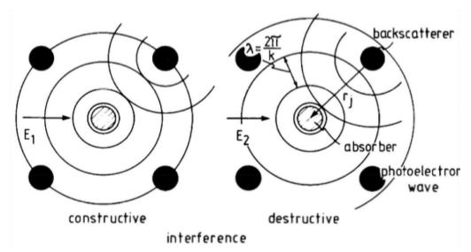
**Figure 3.6** Interference phenomenon between outgoing photoelectron wave and backscattered wave.
