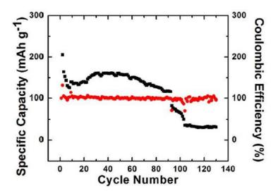
**Figure 6.8** Cycling performance of ZnSnO<sub>3</sub> in NIB system at 240 mA g<sup>-1</sup> without FEC additives.
