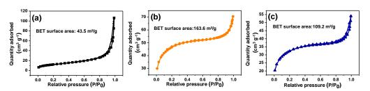
Figure 5.5 N<sub>2</sub> adsorption/desorption BET measurements of (a) pristine SnO<sub>2</sub> (b)
