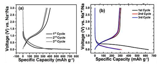
**Figure 7.4** Sodiation galvanostatic charge-discharge at a current density of 30 mA g<sup>-1</sup> of (a) laser pyrolyzed pristine SnO<sub>2</sub> (b) ZnSnO<sub>3</sub> hollow cubes
