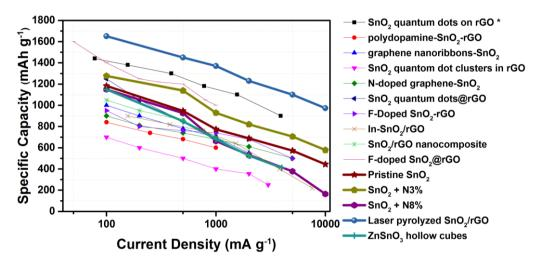
**Figure 7.1** Specific capacity vs. current density plot of the lithiation performance of different graphene-SnO<sub>2</sub> based nanocomposites. \* indicates capacity calculated from SnO<sub>2</sub> only instead of the nanocomposites
