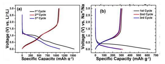
**Figure 6.5** Initial galvanostatic charge-discharge curves of  $ZnSnO_3$  in (a) LIB at 100 mA  $g^{-1}$  (b) NIB at 30 mA  $g^{-1}$
