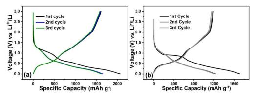
**Figure 4.9** Galvanostatic charge-discharge profiles of (a) rGO-SnO<sub>2</sub> nanocomposite and (b) pristine SnO<sub>2</sub> in LIB at a current of 100 mA g<sup>-1</sup>. Specific capacities were calculated using the total mass in SnO<sub>2</sub>/rGO-SnO<sub>2</sub>.
