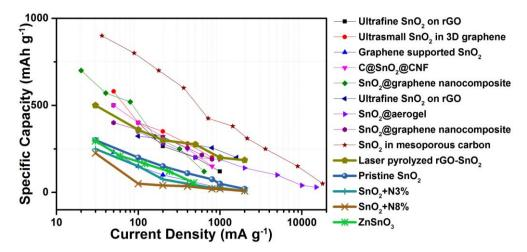
**Figure 7.2** Specific capacity vs. current density plot of the sodiation performance of different carbon- $SnO_2$  based nanocomposites. Reference specific capacities are calculated from  $SnO_2$  only. The specific capacity of laser pyrolyzed  $SnO_2$  is calculated from the mass of composite.
