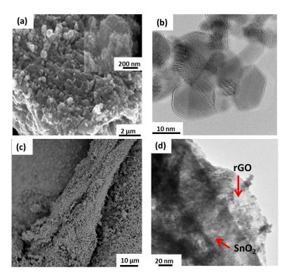
**Figure 4.4** Scanning electron microscope (SEM) and transmission electron microscope (TEM) of (a-b) pristine SnO<sub>2</sub> (c-d) rGO-SnO<sub>2</sub>. Inset in (a) is a magnified view of the SnO<sub>2</sub> nano particulates
