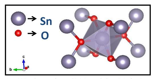
Figure 2.3 Crystal structure of tetragonal SnO<sub>2</sub> (generated using VESTA software)
