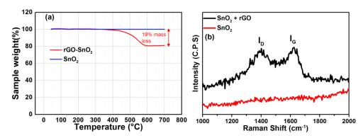
**Figure 4.5** (a) Thermogravimetric analysis (TGA) and (b) Raman spectroscopy of  $SnO_2$  and  $rGO-SnO_2$
