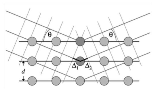
**Figure 3.4** Illustration of the Bragg's diffraction that correlates with the equation  $n\lambda = 2d\sin\theta^4$
