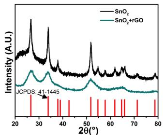
**Figure 4.3** XRD pattern of pristine SnO<sub>2</sub> and rGO-SnO<sub>2</sub> prepared using Sn(OH)<sub>4</sub> as precursor.
