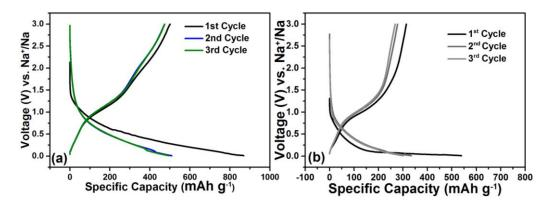
**Figure 4.10** Galvanostatic charge-discharge profiles of (a) rGO-SnO<sub>2</sub> nanocomposite and (b) pristine SnO<sub>2</sub> in NIB at a current of 30 mA g<sup>-1</sup> Specific capacities were calculated using the total mass in SnO<sub>2</sub>/rGO-SnO<sub>2</sub>.
