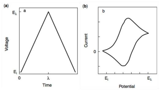
**Figure 3.8** (a) Linear increase in potential with respect to time that is commonly used in CV experiments. (b) The corresponding current response during voltage sweep in CV with respect to the applied potential.<sup>7</sup>
