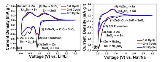
**Figure 6.4** Cyclic voltammogram of ZnSnO<sub>3</sub> under a scan rate of 0.1 mV s<sup>-1</sup> in (a) LIB and (b) NIB.
