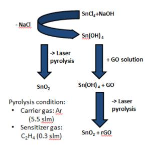
Figure 4.2 Flow diagram illustrating the synthesis pathway for SnO<sub>2</sub> and rGO-SnO<sub>2</sub>
