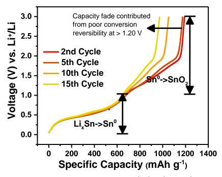
**Figure 7.5** Charge profile of  $SnO_2+N3\%$ , in the  $2^{nd}$ ,  $5^{th}$ ,  $10^{th}$  and  $15^{th}$  cycle. Capacity loss can be seen from lower capacity contribution > 1.20V, indicating poor reversibility of conversion reaction. The alloying process, on the other hand, showed almost perfect capacity retention within the 15 cycles.
