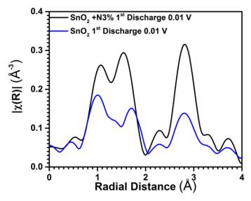
**Figure 5.13** Comparison of EXAFS data for undoped SnO<sub>2</sub> against SnO<sub>2</sub>+N3% at full discharge 0.01 V vs. Li<sup>+</sup>/Li
