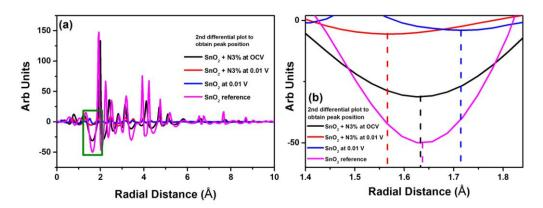
**Figure 5.14** (a)  $2^{nd}$  order differential EXAFS results comparing  $SnO_2$  and  $SnO_2 + N3\%$ . The peak positions could be reliably compared using the differential plots. The area boxed in green between 1.4 to 1.8 Å is magnified and illustrated in (b).
