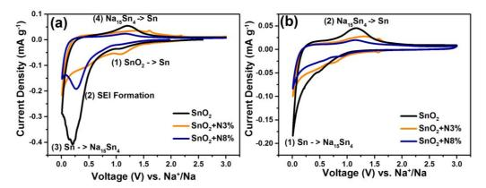
**Figure 5.7** (a)  $1^{st}$  and (b)  $2^{nd}$  sodiation cycle CV curves for the laser pyrolysed samples at 0.1 mV s<sup>-1</sup>. Sharp peak at ~0.6 V corresponds formation of SEI layer on the surface of the electrode during the initial discharge process.
