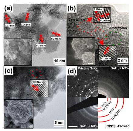
**Figure 5.2** HRTEM images of (a) pristine SnO<sub>2</sub> (b) SnO<sub>2</sub>-N3%, and (c) SnO<sub>2</sub>-N8%. The insets display the corresponding FESEM images and the inverse FFT images after applying an array mask. Samples prepared under the presence of NH<sub>3</sub> displays polycrystalline behavior along with grains of crystalline and amorphous regions. The
