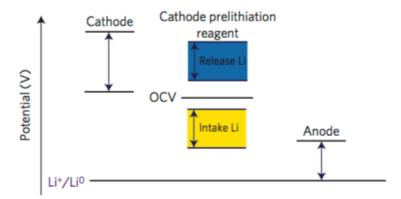
Figure 7.7 Potential requirements for the ideal cathode additives<sup>8</sup>
