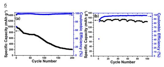
**Figure 6.7** Cycling performance of ZnSnO<sub>3</sub> within a voltage window of 0.01 to 3.00 V vs. Li<sup>+</sup>/Li or Na<sup>+</sup>/Na in (a) LIB at 100 mA g<sup>-1</sup> and (b) NIB at 240 mA g<sup>-1</sup>
