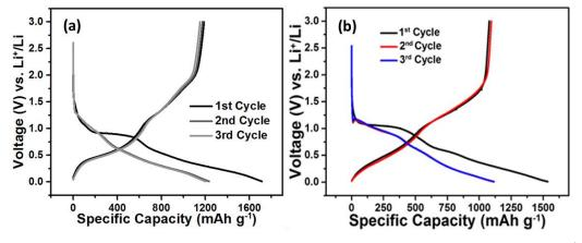
**Figure 7.3** Lithiation galvanostatic charge-discharge at a current density of 100 mA g<sup>-1</sup> of (a) laser pyrolyzed pristine SnO<sub>2</sub> (b) ZnSnO<sub>3</sub> hollow cubes
