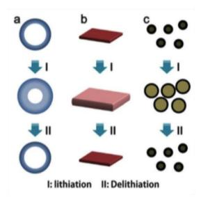
**Figure 2.4** Commonly utilized design structures for alleviating pulverization effect of SnO<sub>2</sub> nanomaterials. (a) hollow structure (b) 2D- nanosheets structure (c) amorphous carbon coating<sup>60</sup>
