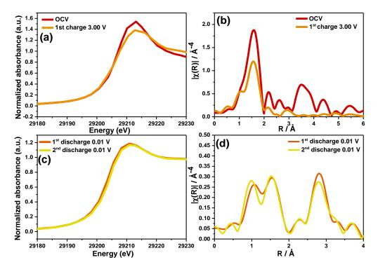
**Figure 5.15** Sn K-edge (a) XANES normalized absorption and (b) Fourier transformed EXAFS spectrums for  $SnO_2+N3\%$  during OCV and after  $1^{st}$  charge at 3.00 V. (c) & (d) similarly corresponds to the XANES and FT EXAFS at 0.01 V during full discharge in the  $1^{st}$  and  $2^{nd}$  cycle.
