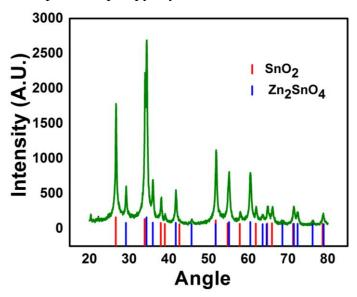
**Figure 7.6** XRD spectrum of laser pyrolyzed product utilizing SnSO<sub>4</sub> and ZnCl<sub>2</sub> as initial precursors.
