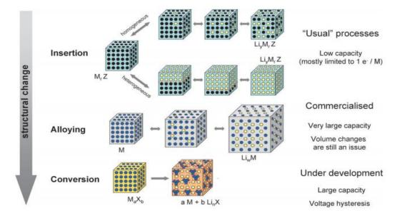
**Figure 2.2** Schematic representing the different reaction mechanisms of electrode materials in alkali ion batteries<sup>7</sup>
