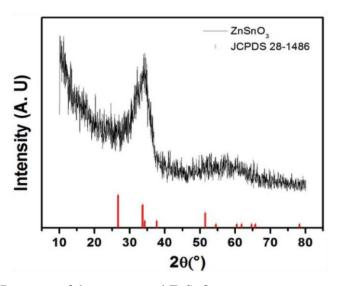
Figure 6.1 XRD pattern of the as-prepared ZnSnO<sub>3</sub>
