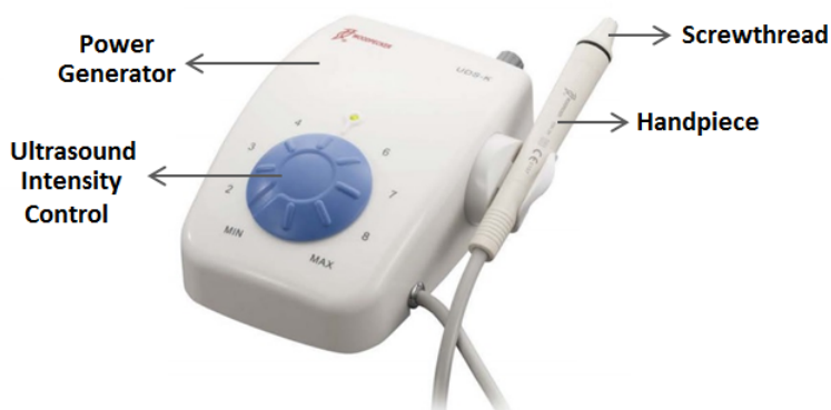
Figure 5.1: Dental scaler used as the sonicator in this research.
