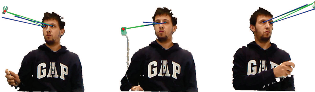
Figure 4.15: Some results of the final gaze estimation using our feature-based system. The green lines define the ground truth and blue lines represent the estimation, the red point shows the tracked object.
